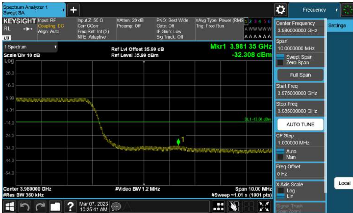
Sub6 n77(78). High Band Edge Plot (30 M BW Ch.664332 BPSK FullRB)(1)
