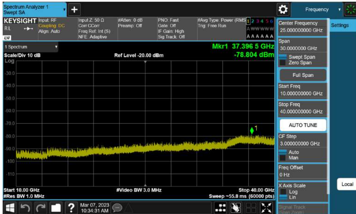
Sub6 n77(78). Conducted Spurious Plot_2 (648000ch_40 MHz_BPSK)
