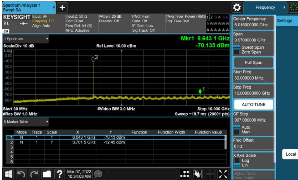
Sub6 n77(78). Conducted Spurious Plot_1 (648000ch_40 MHz_BPSK)
