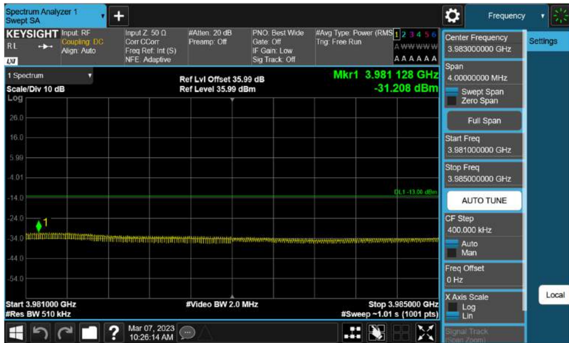
Sub6 n77(78). High Band Edge Plot (30 M BW Ch.664332 BPSK FullRB)(2)
