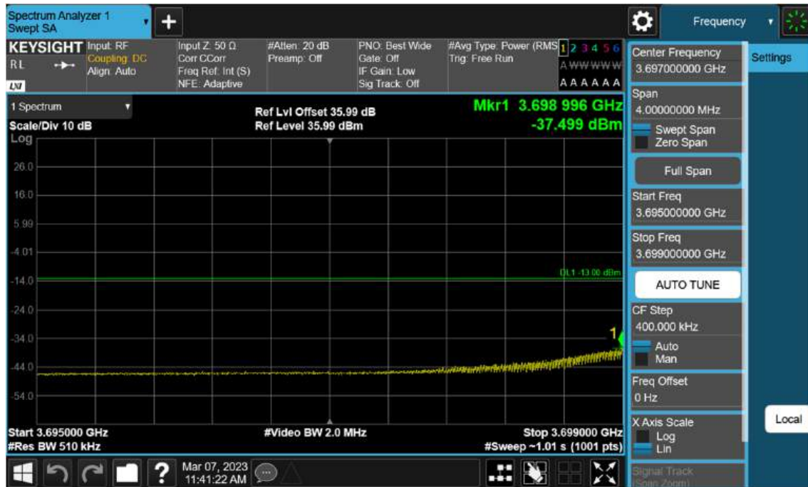
Sub6 n77(78). Low Band Edge Plot (70 M BW Ch.649000 BPSK 1RB)(2)
