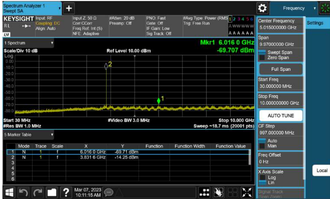
Sub6 n77(78). Conducted Spurious Plot_1 (656000ch_20 MHz_BPSK)
