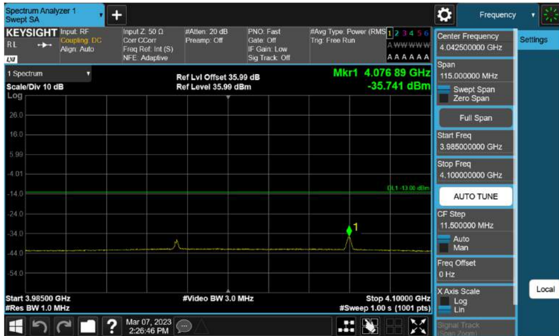
Sub6 n77(78). High Band Edge Plot (100 M BW Ch.662000 BPSK 1RB)(3)
