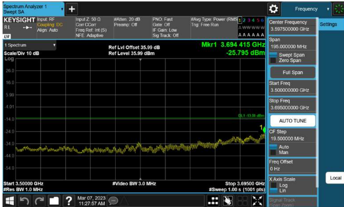
Sub6 n77(78). Low Band Edge Plot (60 M BW Ch.648668 BPSK FullRB)(3)
