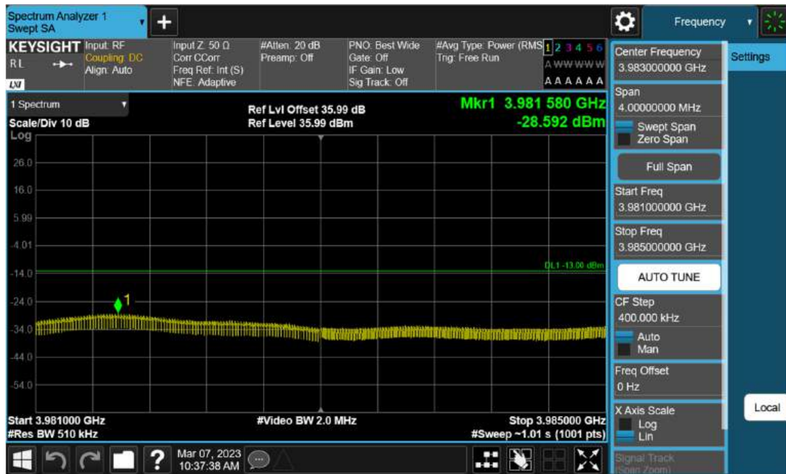
Sub6 n77(78). High Band Edge Plot (40 M BW Ch.664000 BPSK FullRB)(2)
