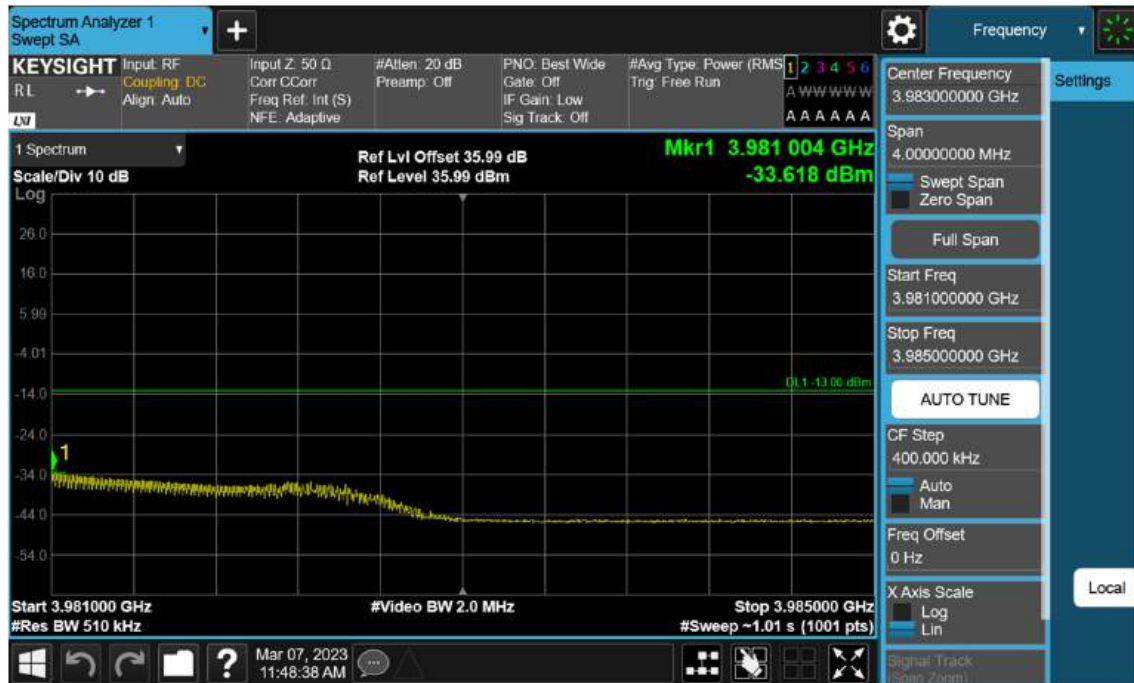
Sub6 n77(78). High Band Edge Plot (70 M BW Ch.663000 BPSK 1RB)(2)
