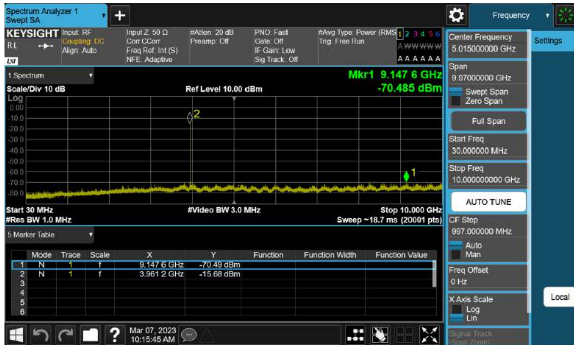
Sub6 n77(78). Conducted Spurious Plot_1 (664666ch_20 MHz_BPSK)
