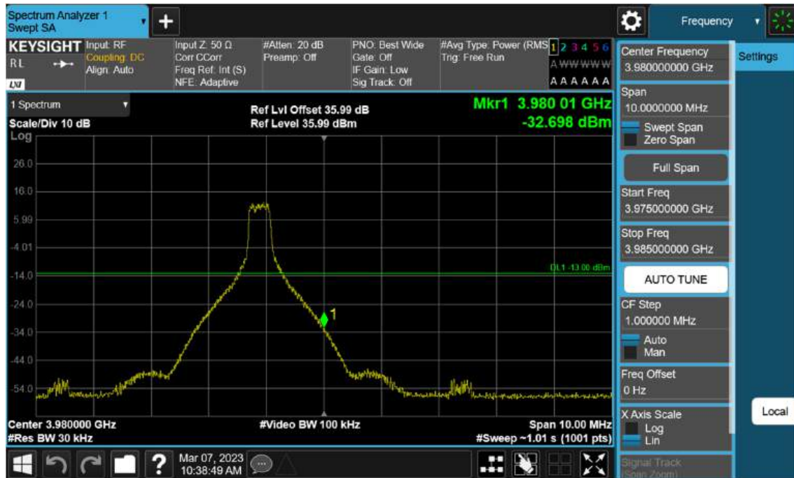
Sub6 n77(78). High Band Edge Plot (40 M BW Ch.664000 BPSK 1RB)(1)
