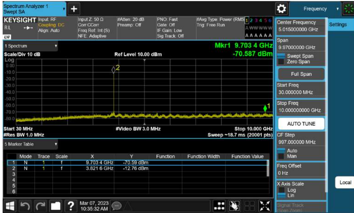
Sub6 n77(78). Conducted Spurious Plot_1 (656000ch_40 MHz_BPSK)
