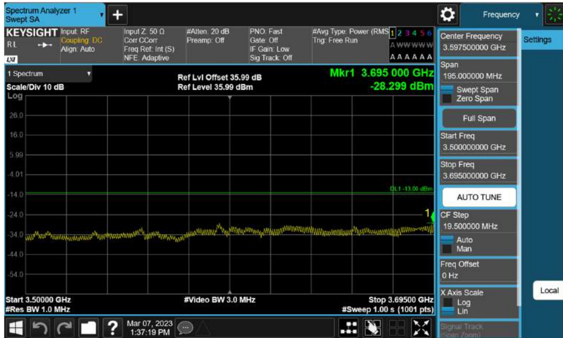
Sub6 n77(78). Low Band Edge Plot (90 M BW Ch.649668 BPSK FullRB)(3)
