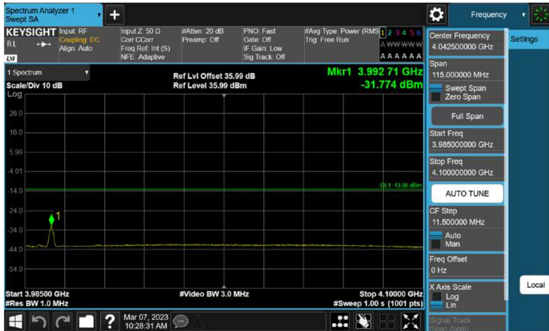
Sub6 n77(78). High Band Edge Plot (30 M BW Ch.664332 BPSK 1RB)(3)
