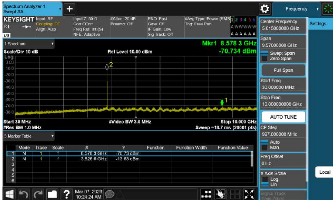
Sub6 n77(78). Conducted Spurious Plot_1 (656000ch_30 MHz_BPSK)
