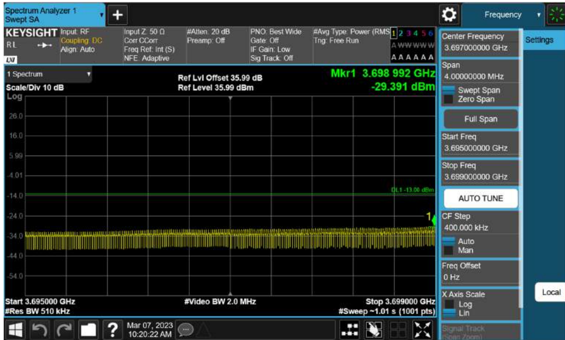
Sub6 n77(78). Low Band Edge Plot (30 M BW Ch.647668 BPSK FullRB)(2)
