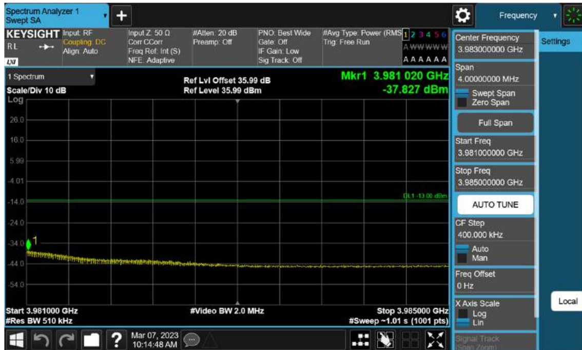
Sub6 n77(78). High Band Edge Plot (20 M BW Ch.664666 BPSK 1RB)(2)
