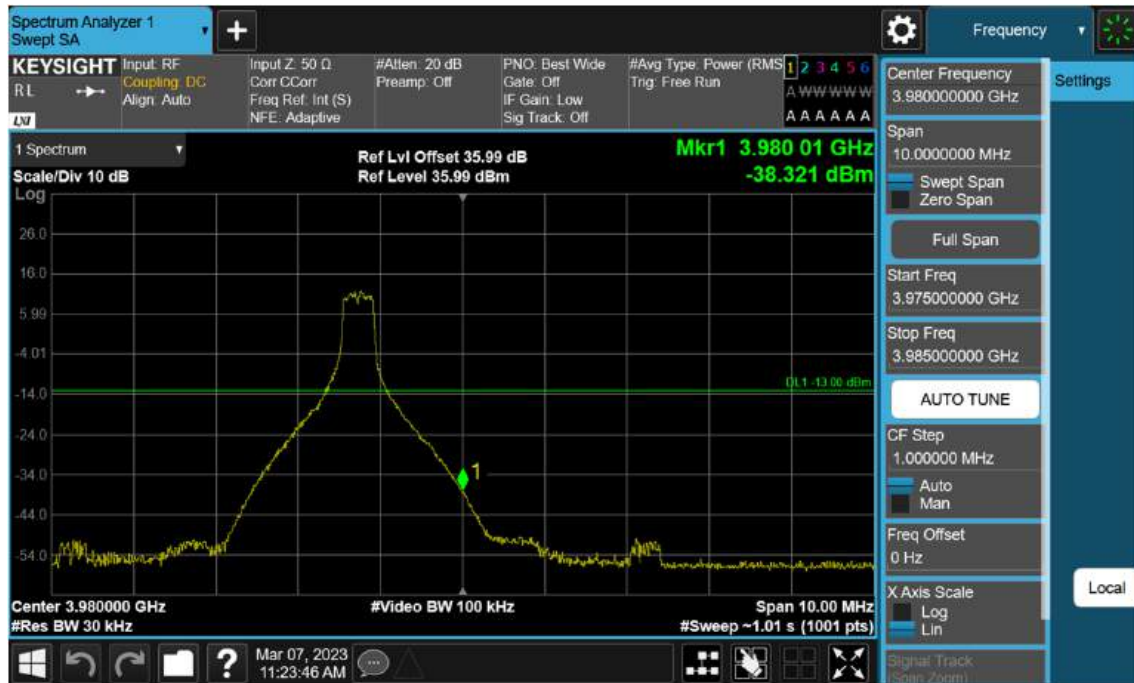
Sub6 n77(78). High Band Edge Plot (50 M BW Ch.663666 BPSK 1RB)(1)
