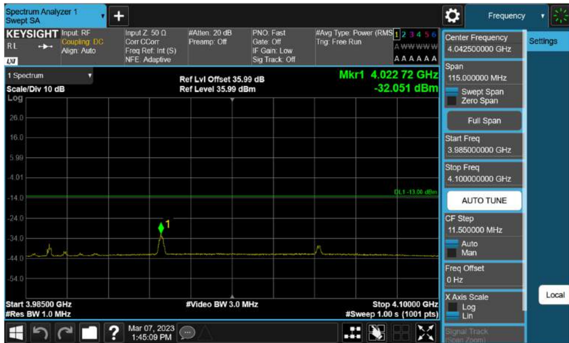
Sub6 n77(78). High Band Edge Plot (90 M BW Ch.662332 BPSK 1RB)(3)
