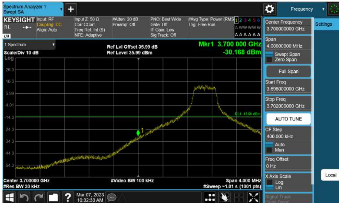
Sub6 n77(78). Low Band Edge Plot (40 M BW Ch.648000 BPSK 1RB)(1)
