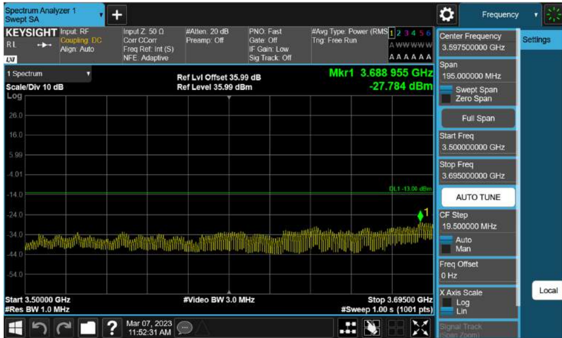
Sub6 n77(78). Low Band Edge Plot (80 M BW Ch.649334 BPSK FullRB)(3)
