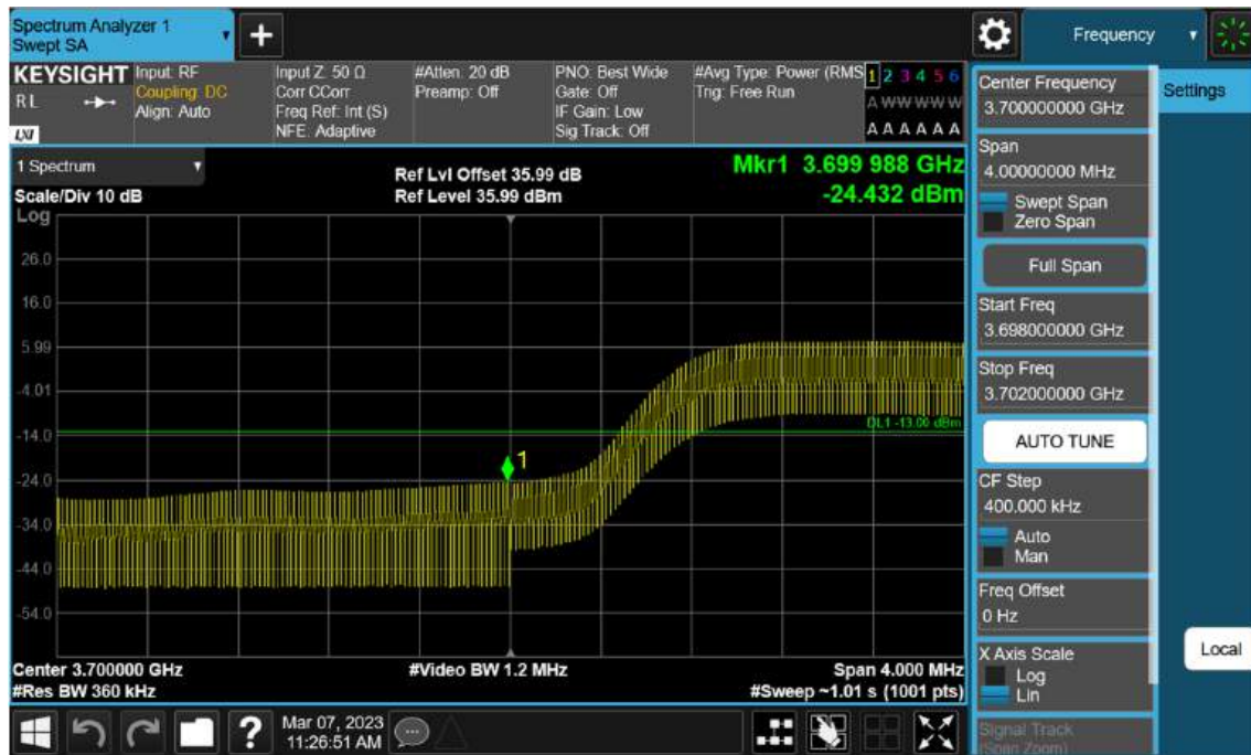
Sub6 n77(78). Low Band Edge Plot (60 M BW Ch.648668 BPSK FullRB)(1)
