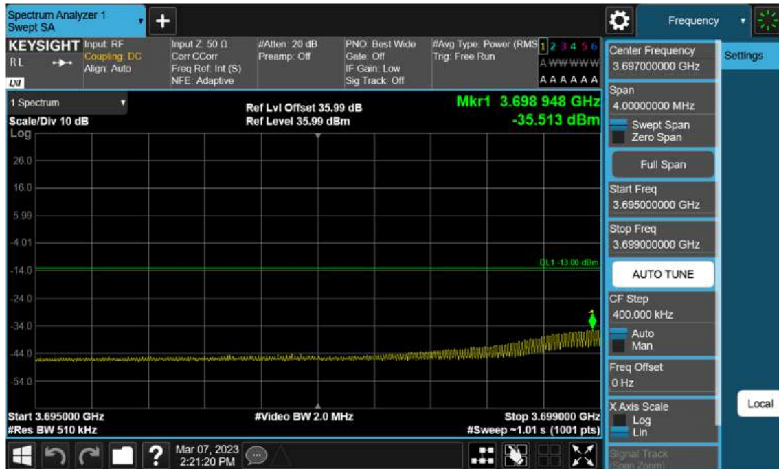
Sub6 n77(78). Low Band Edge Plot (100 M BW Ch.650000 BPSK 1RB)(2)
