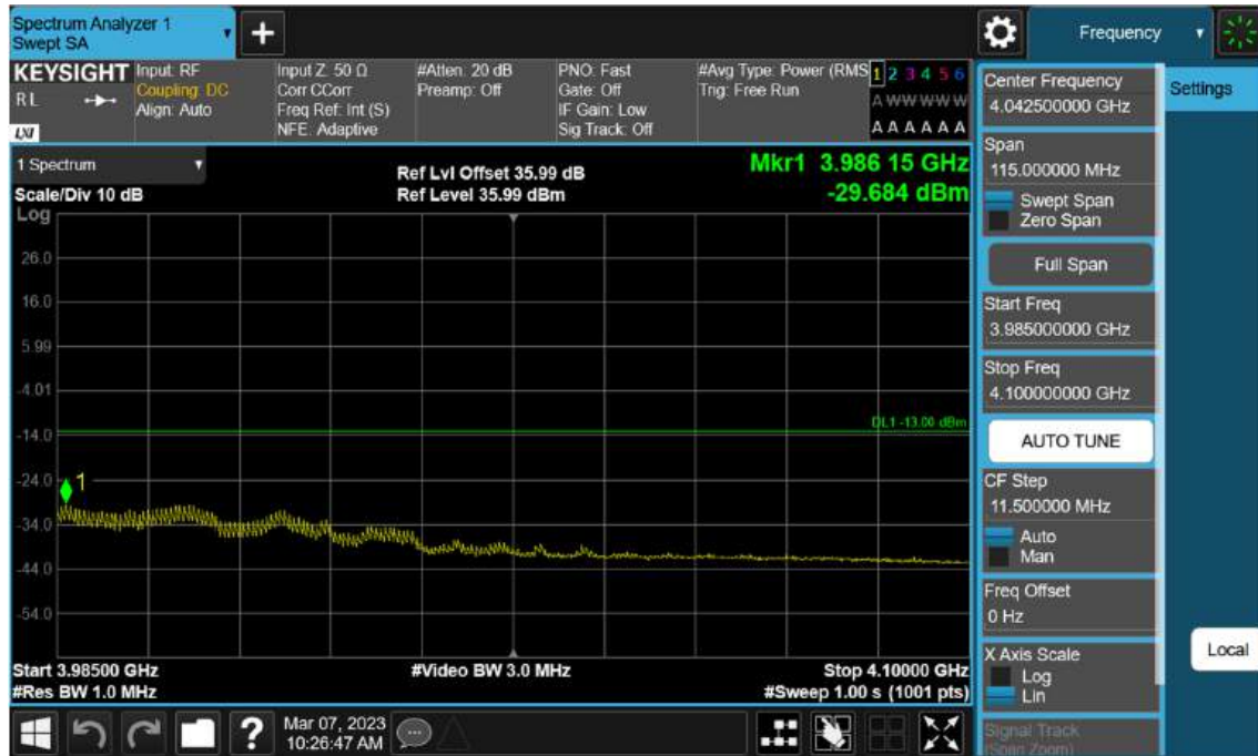
Sub6 n77(78). High Band Edge Plot (30 M BW Ch.664332 BPSK FullRB)(3)
