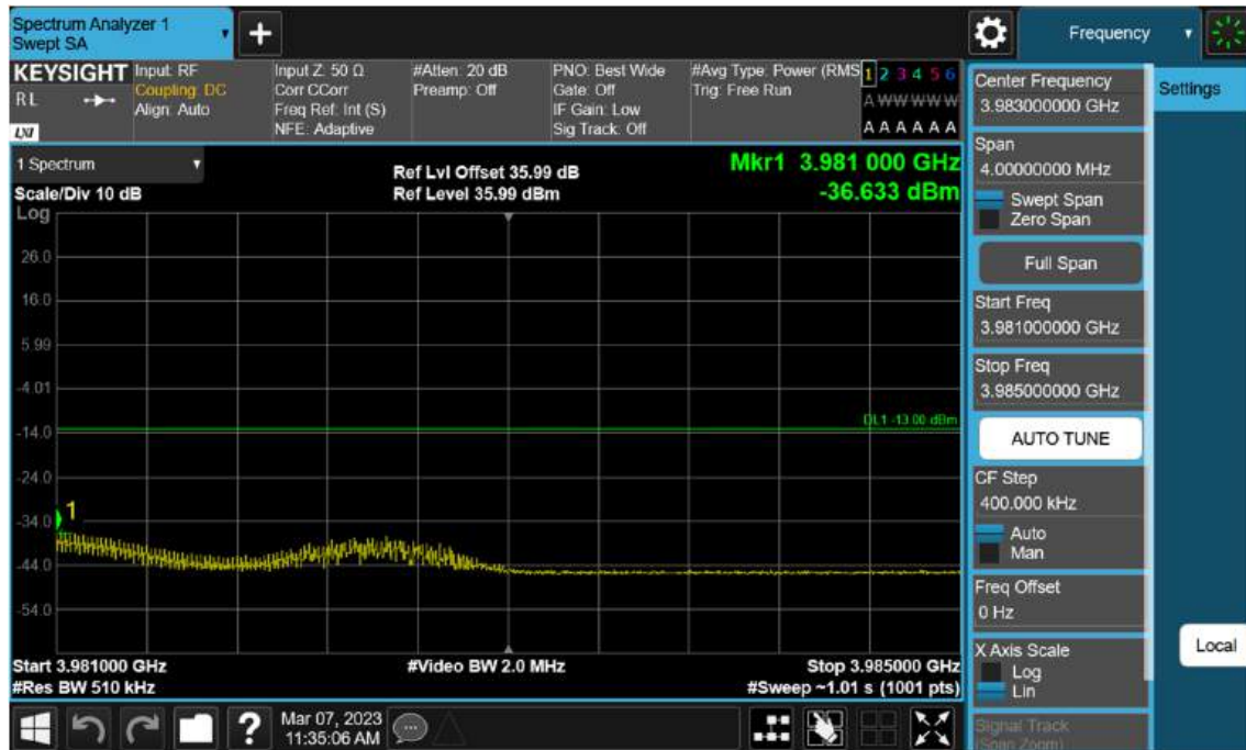
Sub6 n77(78). High Band Edge Plot (60 M BW Ch.663332 BPSK 1RB)(2)
