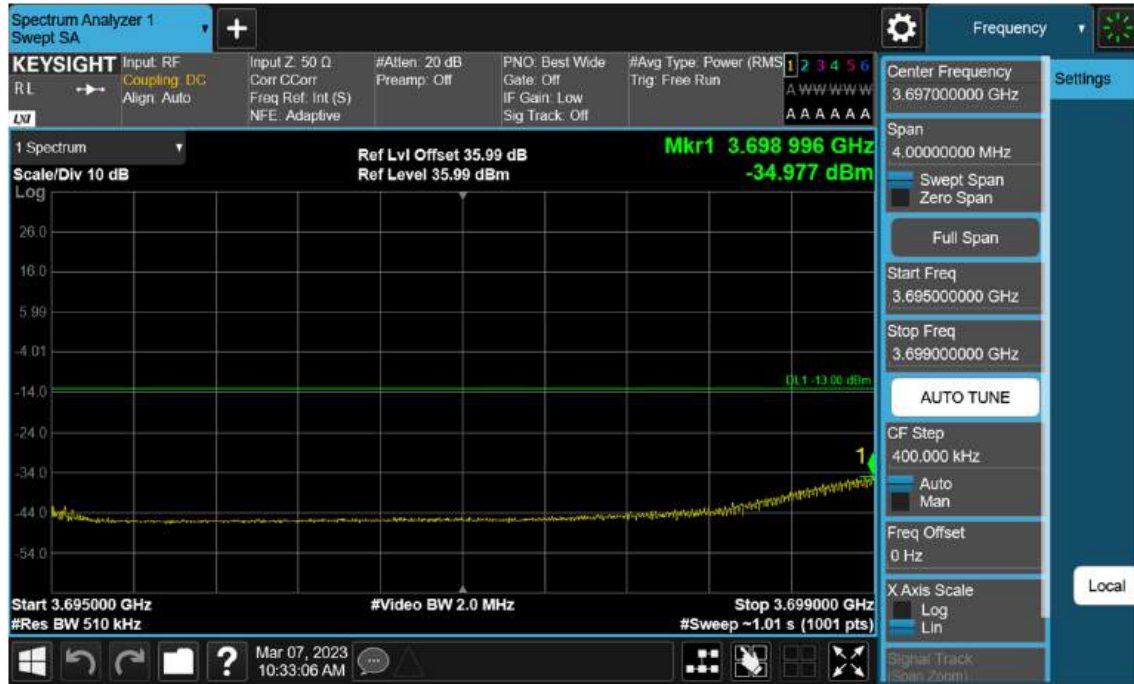
Sub6 n77(78). Low Band Edge Plot (40 M BW Ch.648000 BPSK 1RB)(2)
