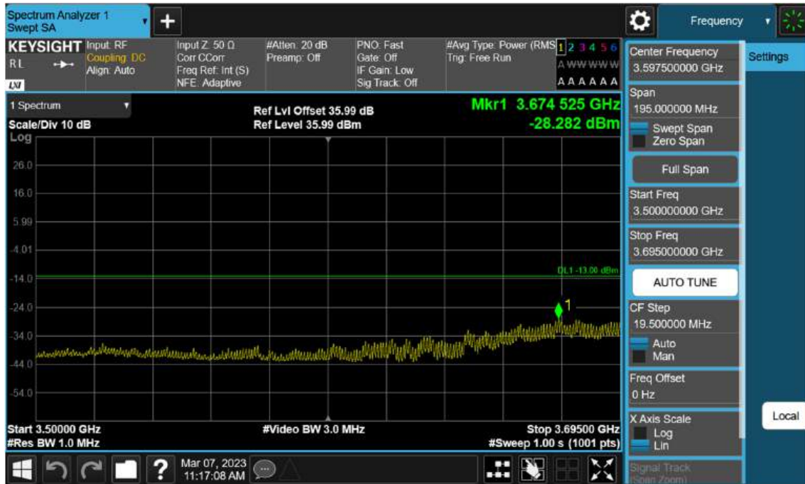
Sub6 n77(78). Low Band Edge Plot (50 M BW Ch.648334 BPSK FullRB)(3)
