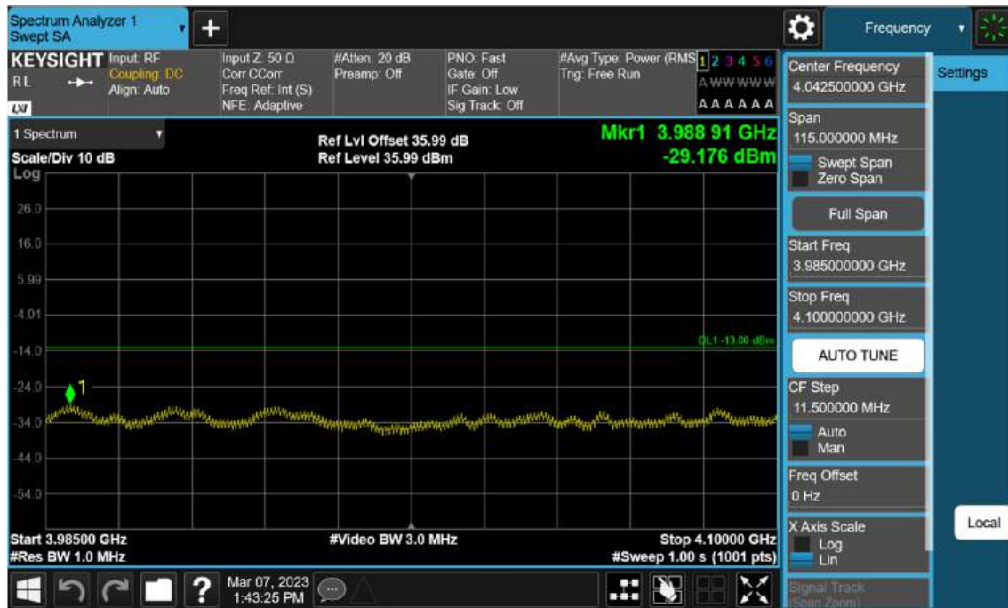
Sub6 n77(78). High Band Edge Plot (90 M BW Ch.662332 BPSK FullRB)(3)
