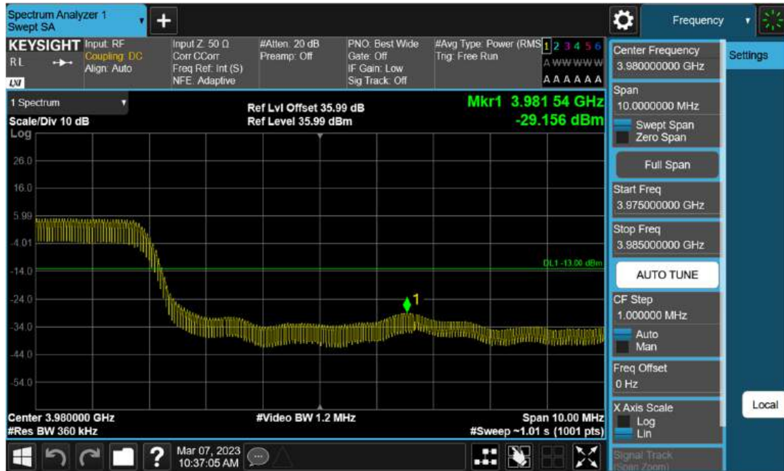
Sub6 n77(78). High Band Edge Plot (40 M BW Ch.664000 BPSK FullRB)(1)
