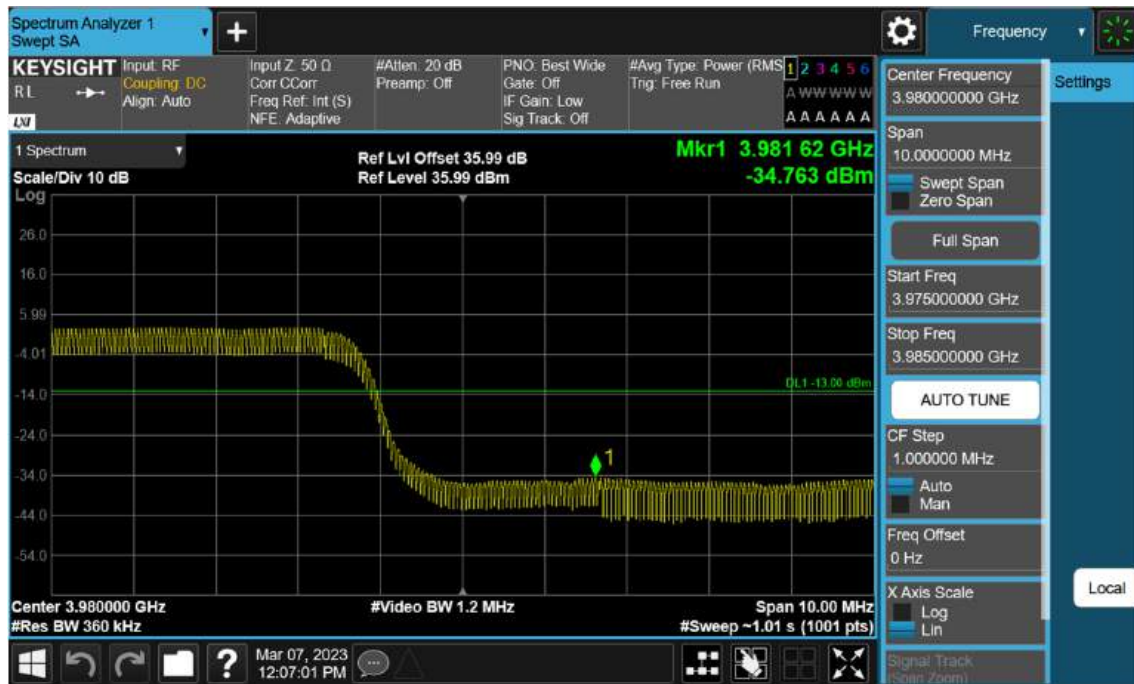
Sub6 n77(78). High Band Edge Plot (80 M BW Ch.662666 BPSK FullRB)(1)
