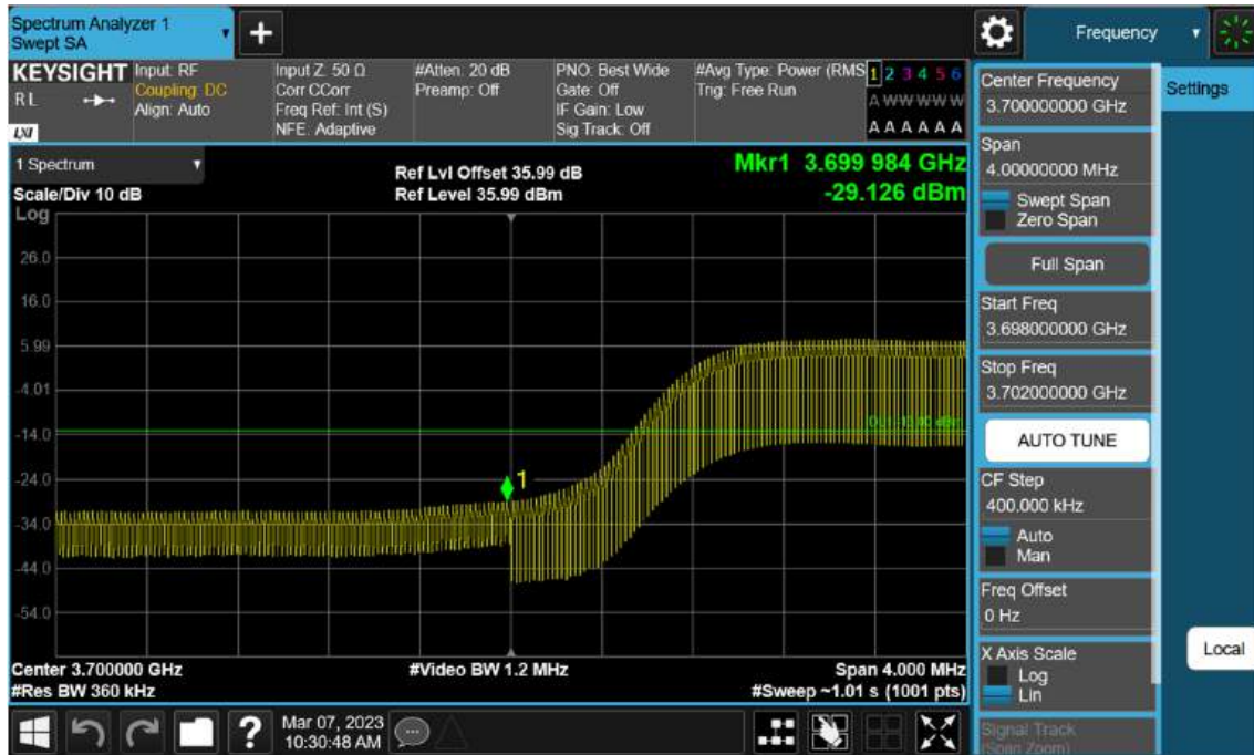
Sub6 n77(78). Low Band Edge Plot (40 M BW Ch.648000 BPSK FullRB)(1)
