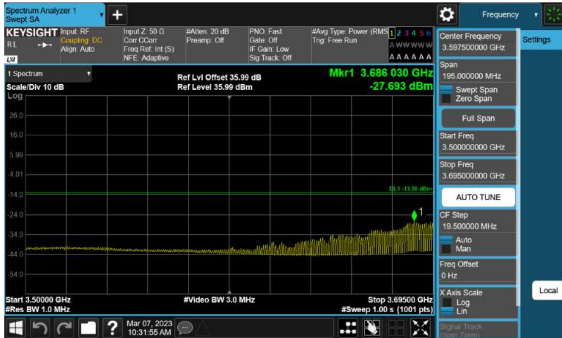
Sub6 n77(78). Low Band Edge Plot (40 M BW Ch.648000 BPSK FullRB)(3)
