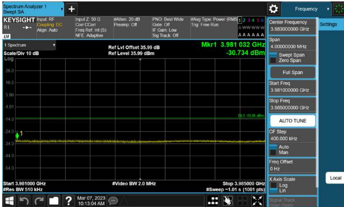
Sub6 n77(78). High Band Edge Plot (20 M BW Ch.664666 BPSK FullRB)(2)
