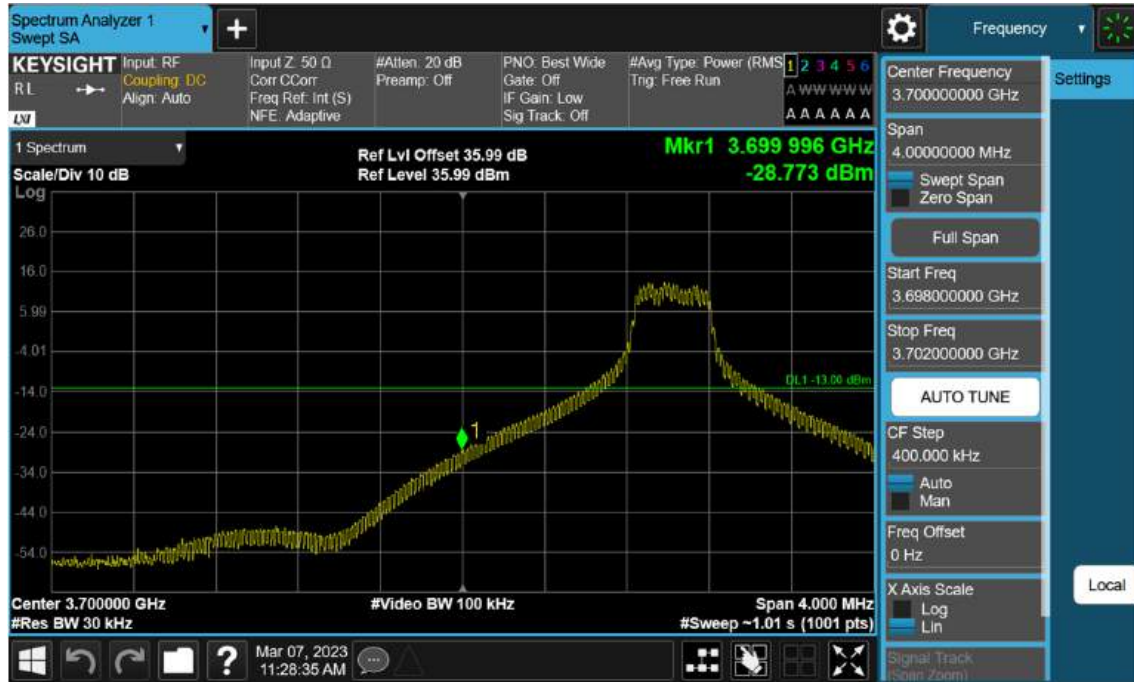
Sub6 n77(78). Low Band Edge Plot (60 M BW Ch.648668 BPSK 1RB)(1)
