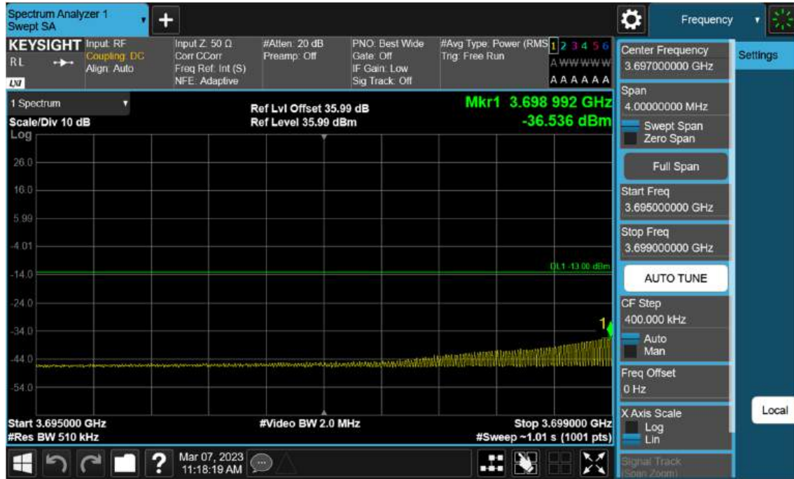
Sub6 n77(78). Low Band Edge Plot (50 M BW Ch.648334 BPSK 1RB)(2)
