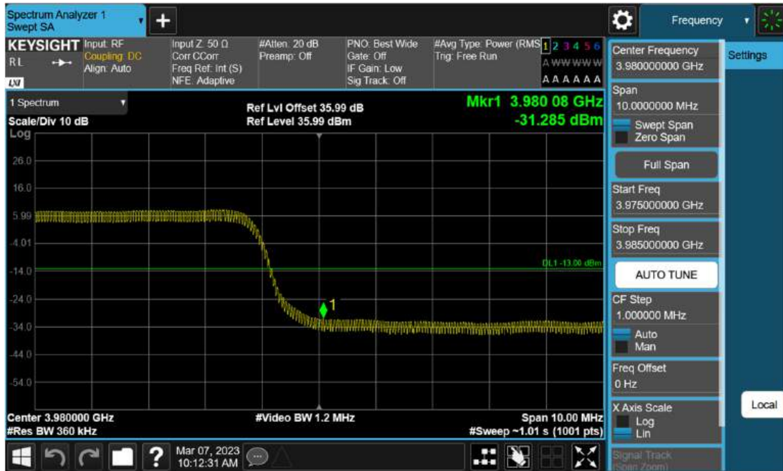
Sub6 n77(78). High Band Edge Plot (20 M BW Ch.664666 BPSK FullRB)(1)
