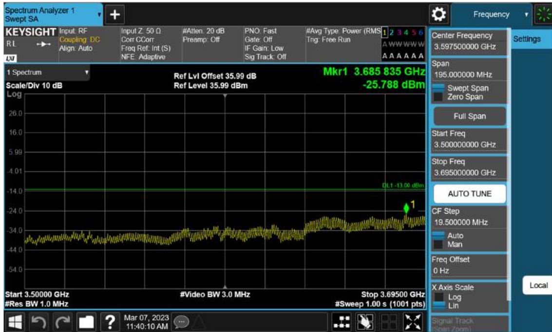
Sub6 n77(78). Low Band Edge Plot (70 M BW Ch.649000 BPSK FullRB)(3)
