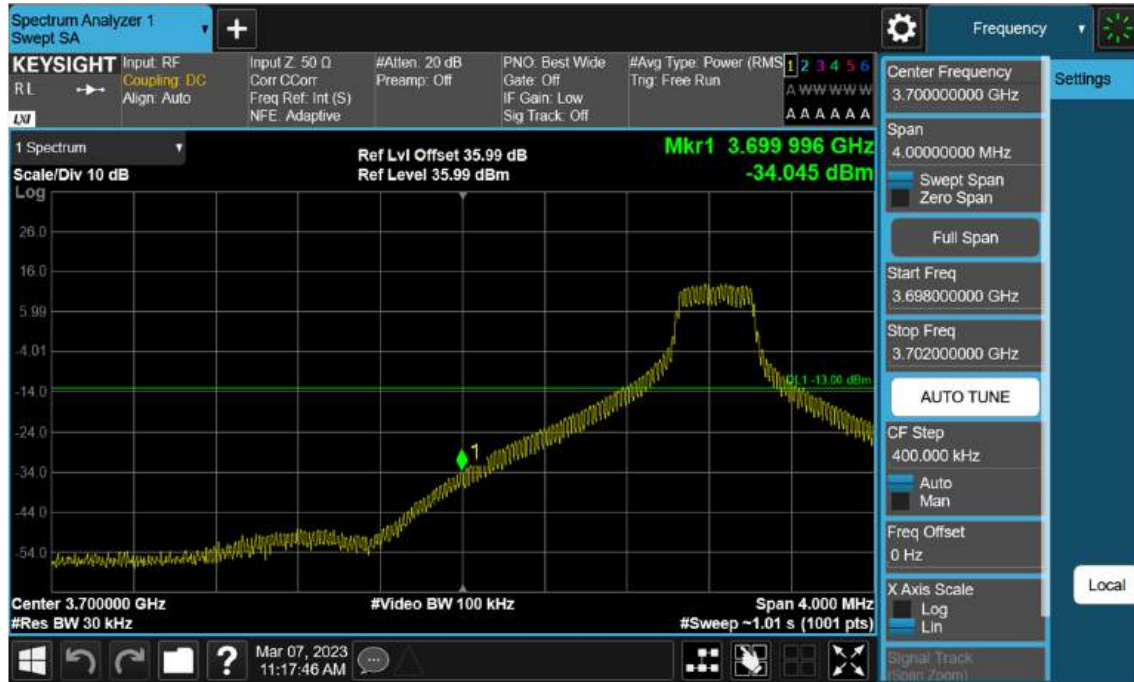
Sub6 n77(78). Low Band Edge Plot (50 M BW Ch.648334 BPSK 1RB)(1)
