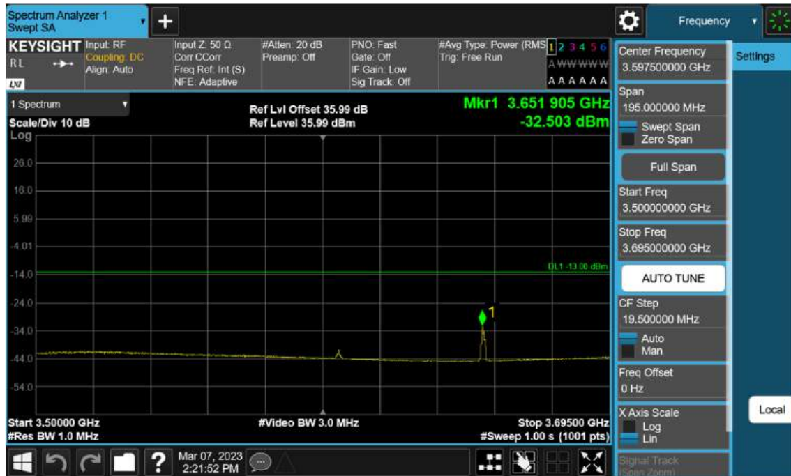
Sub6 n77(78). Low Band Edge Plot (100 M BW Ch.650000 BPSK 1RB)(3)
