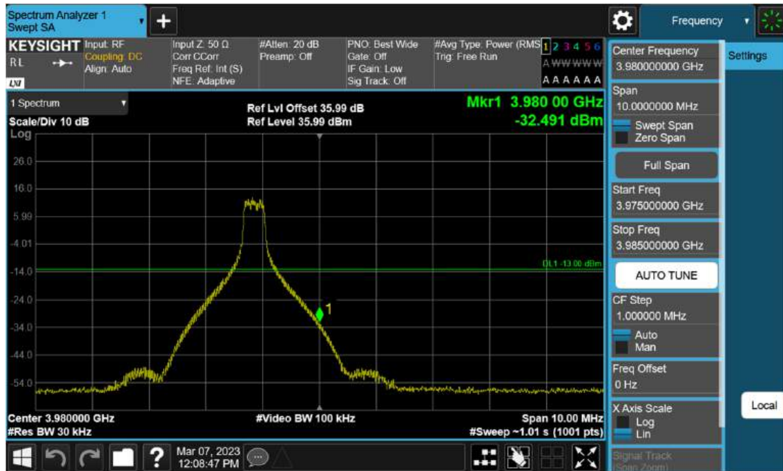
Sub6 n77(78). High Band Edge Plot (80 M BW Ch.662666 BPSK 1RB)(1)
