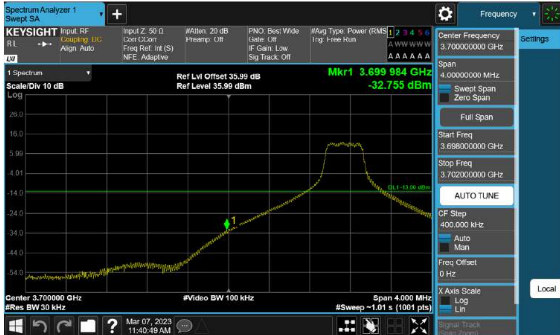
Sub6 n77(78). Low Band Edge Plot (70 M BW Ch.649000 BPSK 1RB)(1)
