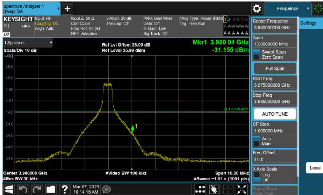
Sub6 n77(78). High Band Edge Plot (20 M BW Ch.664666 BPSK 1RB)(1)
