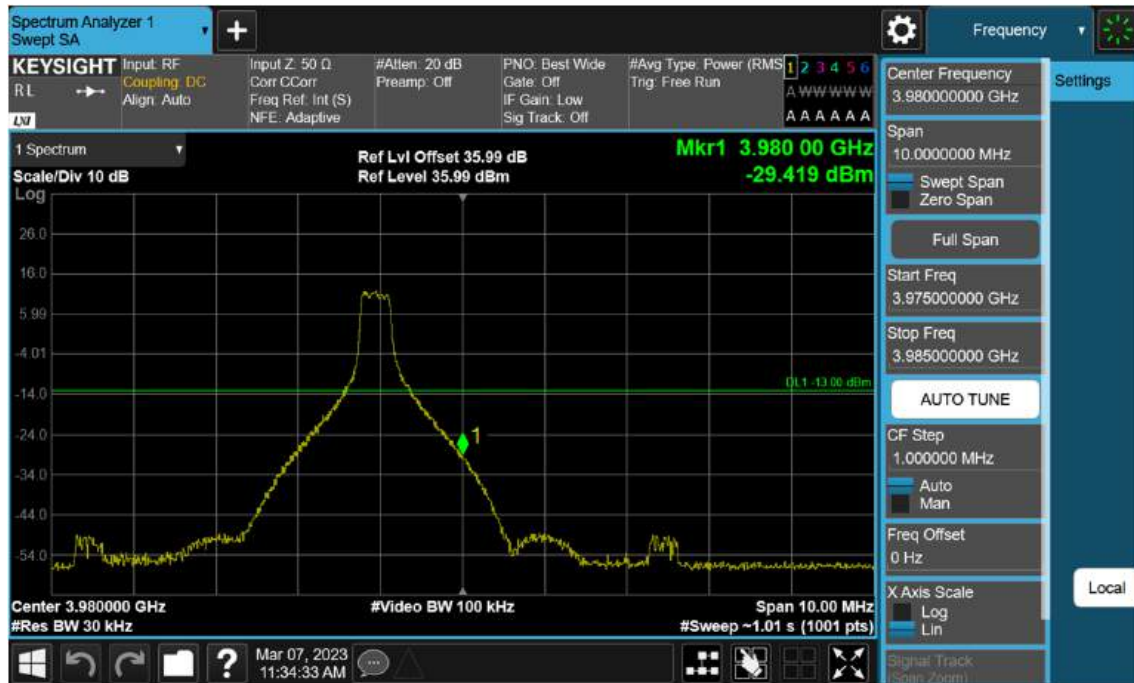
Sub6 n77(78). High Band Edge Plot (60 M BW Ch.663332 BPSK 1RB)(1)
