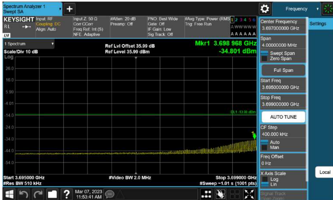
Sub6 n77(78). Low Band Edge Plot (80 M BW Ch.649334 BPSK 1RB)(2)
