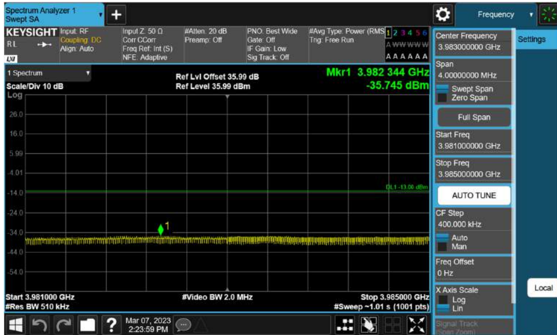
Sub6 n77(78). High Band Edge Plot (100 M BW Ch.662000 BPSK FullRB)(2)
