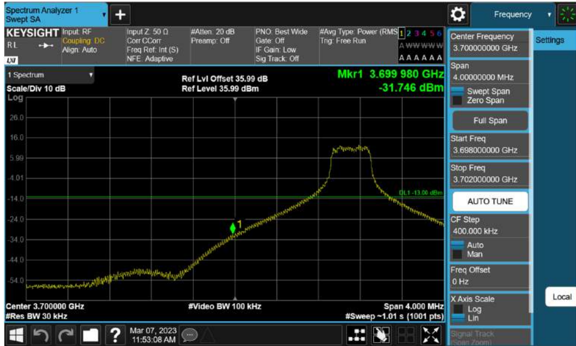
Sub6 n77(78). Low Band Edge Plot (80 M BW Ch.649334 BPSK 1RB)(1)
