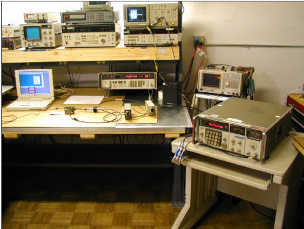
General equipment arrangement for FCC requested re-measurement work, LoJack-03.
