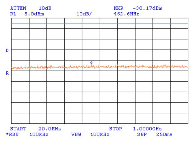
Limit for spurious emissions = – 0.33 dBm No spurious emissions were found
