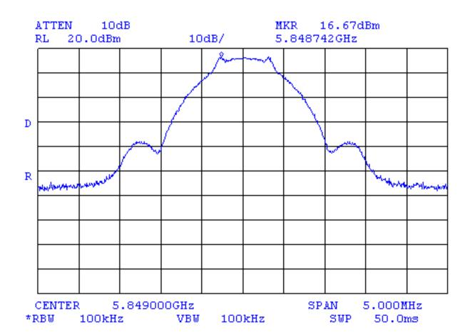
Limit for spurious emissions = 16.67 dBm - 20 dB = -3.33 dBm
