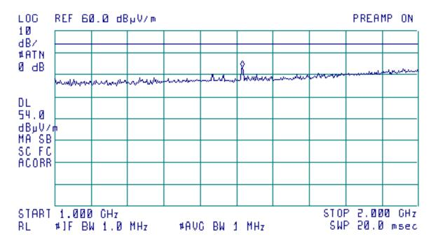
Limit (average) for radiated spurious emissions in restricted bands is 54 dB(μV/m)
