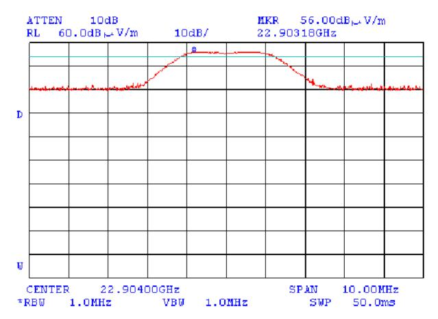
Peak limit for radiated emission is 74 dB( $\mu$ V/m) E<sub>peak</sub> = 56 dB( $\mu$ V/m)
