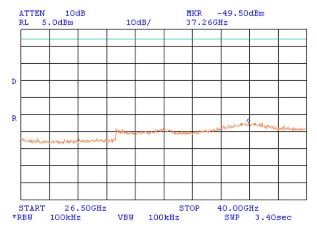
Limit for spurious emissions = – 0.33 dBm No spurious emissions were found
