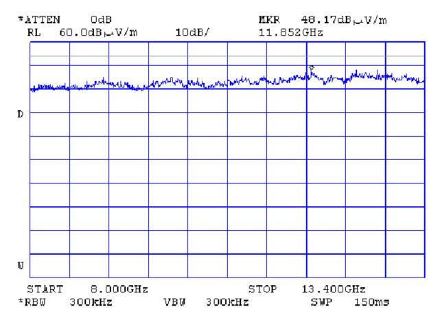
Limit (average) for radiated spurious emissions in restricted bands is 54 dB( $\mu$ V/m)
