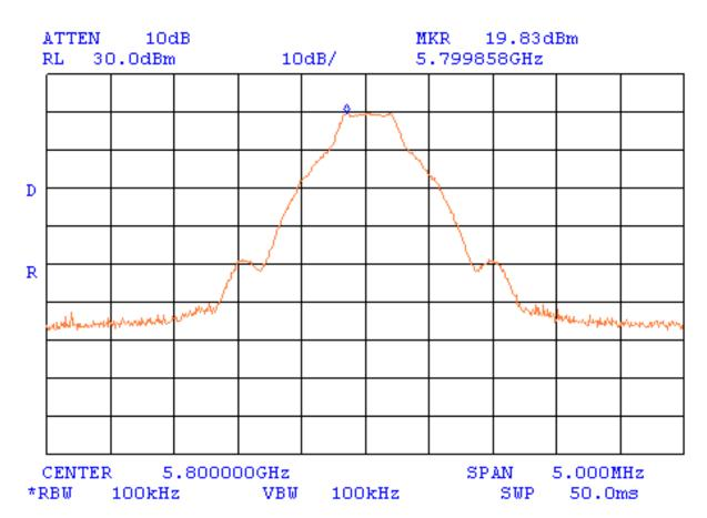
Limit for spurious emissions =19.83 dBm -20 dB = -0.17 dBm
