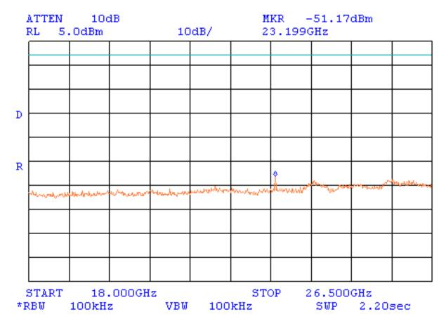
Limit for spurious emissions = – 0.17 dBm No spurious emissions were found
