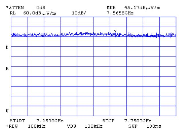
Limit (average) for radiated spurious emissions in restricted bands is 54 dB( $\mu$ V/m) No spurious emissions were found
