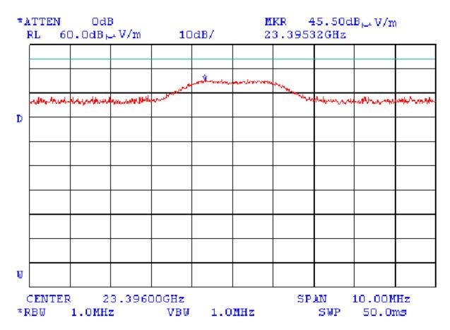
Limit (average) for radiated spurious emissions in restricted bands is 54 dB( $\mu$ V/m) E<sub>peak</sub> = 45.5 dB( $\mu$ V/m)
