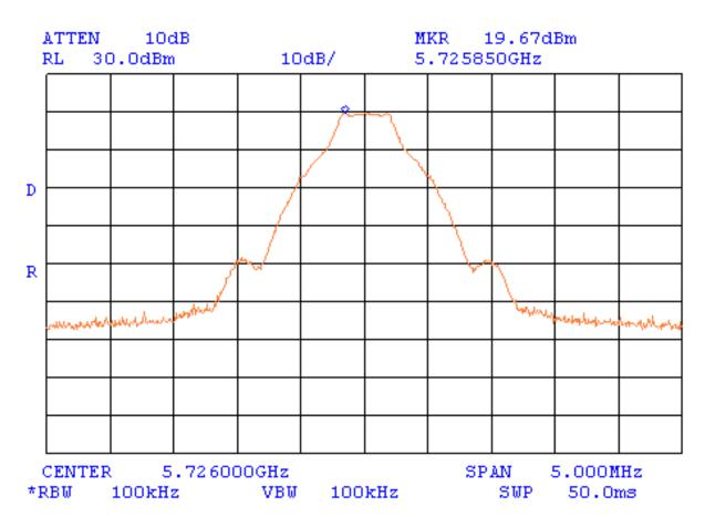
Limit for spurious emissions = 19.67 dBm - 20 dB = -0.33 dBm
