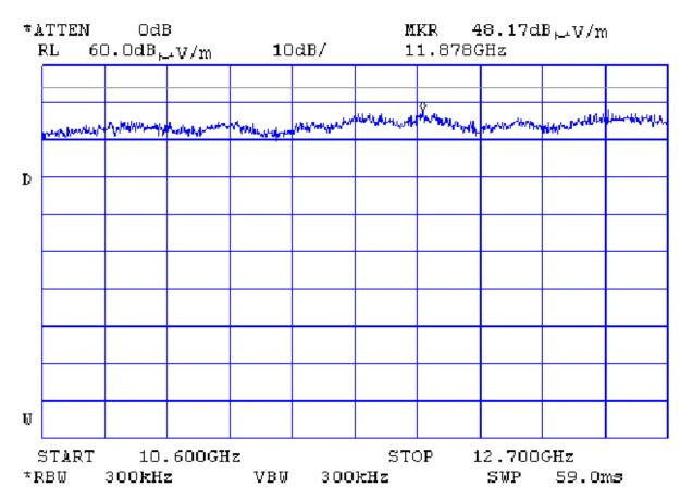
Limit (average) for radiated spurious emissions in restricted bands is 54 dB( $\mu$ V/m)
