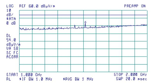
Limit (average) for radiated spurious emissions in restricted bands is 54 dB(µV/m)
