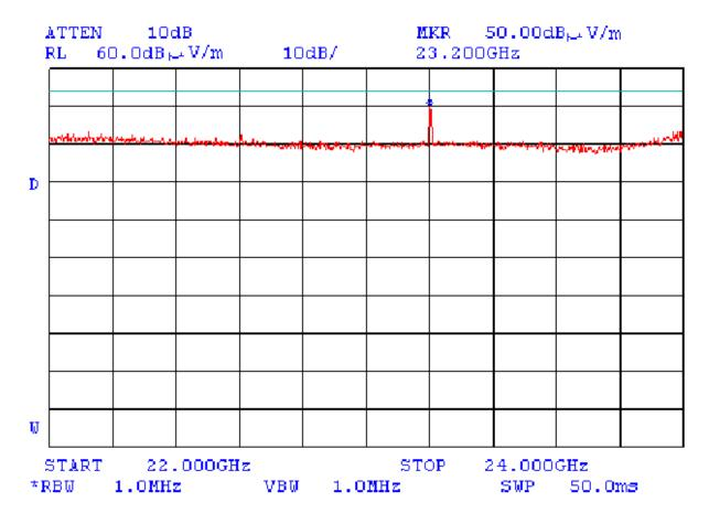
Limit (average) for radiated spurious emissions in restricted bands is 54 dB( $\mu$ V/m) No spurious emissions except 4<sup>th</sup> harmonic were found
