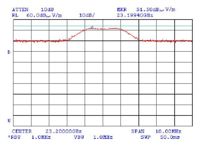
Limit (average) for radiated spurious emissions in restricted bands is 54 dB( $\mu$ V/m) E<sub>peak</sub> = 51.5 dB( $\mu$ V/m)
