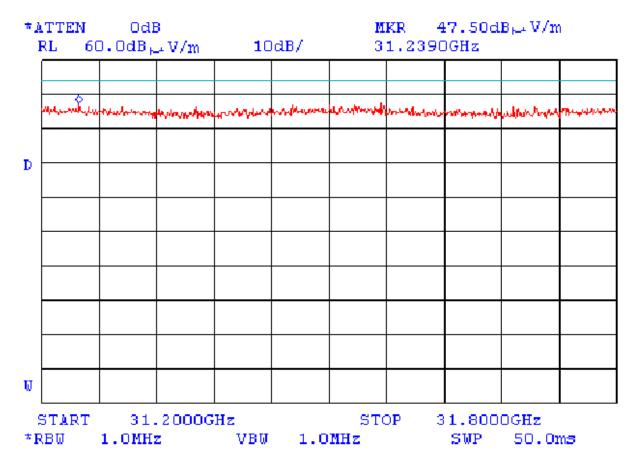
Limit (average) for radiated spurious emissions in restricted bands is 54 dB( $\mu$ V/m) No spurious emissions were found
