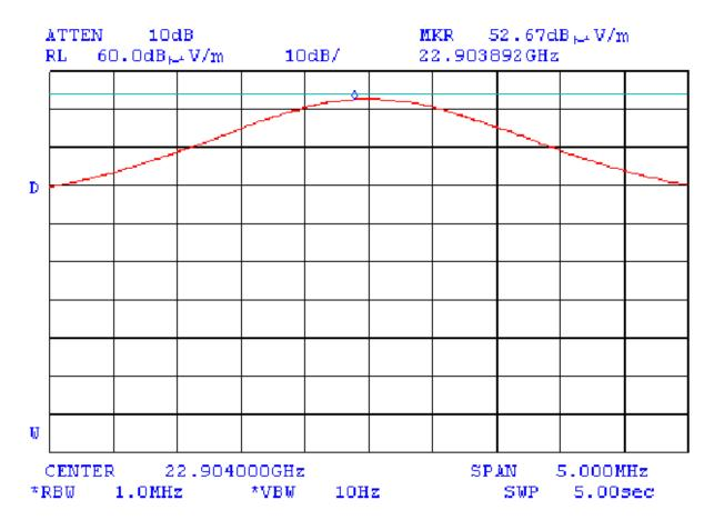
Limit (average) for radiated spurious emissions in restricted bands is 54 dB( $\mu$ V/m) E<sub>aver</sub> = 52.67 dB( $\mu$ V/m)
