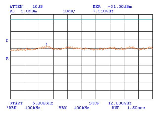
Limit for spurious emissions = – 0.67 dBm No spurious emissions were found
