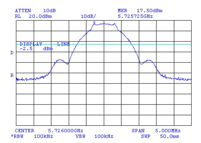
Limit for spurious emissions = 17.5 dBm - 20 dB = -2.5 dBm
