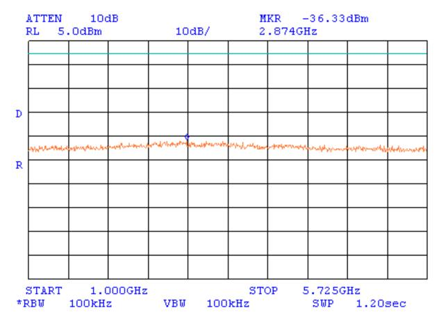
Limit for spurious emissions = – 0.17 dBm No spurious emissions were found
