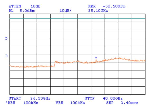
Limit for spurious emissions = – 0.67 dBm No spurious emissions were found
