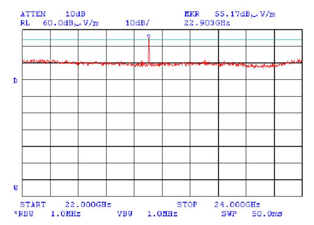
Limit (average) for radiated spurious emissions in restricted bands is 54 dB( $\mu$ V/m) No spurious emissions except 4<sup>th</sup> harmonic were found
