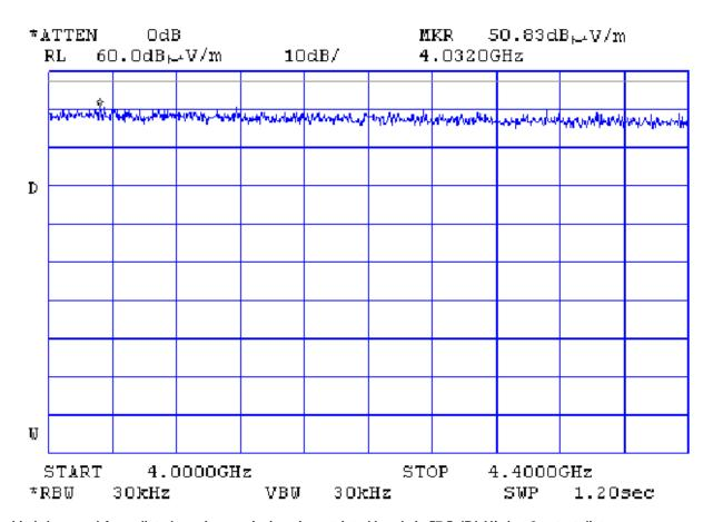
Limit (average) for radiated spurious emissions in restricted bands is 57.5 dB( $\mu$ V/m) at 2 m test distance No spurious emissions were found
