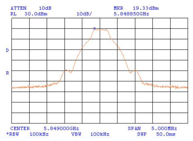
Limit for spurious emissions = 19.33 dBm - 20 dB = -0.67 dBm
