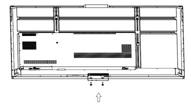
2) Lock the Sensor Box to the bottom of the IFP with screws.
