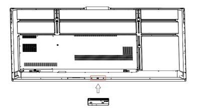
1) Position the Sensor Box to the bottom of the IFP in the direction of the arrow.
