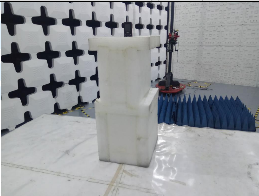
Radiated emission Test Setup (Above 1 GHz)
