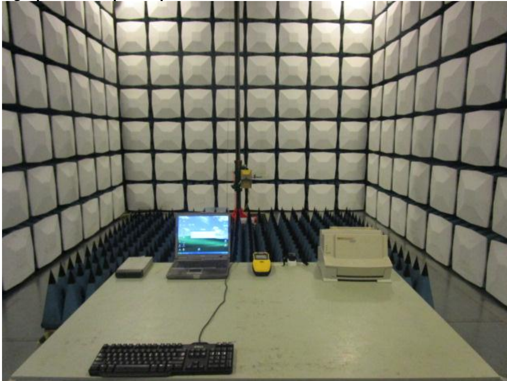
Photograph 3: Set-up for Spurious Emissions above 1GHz
