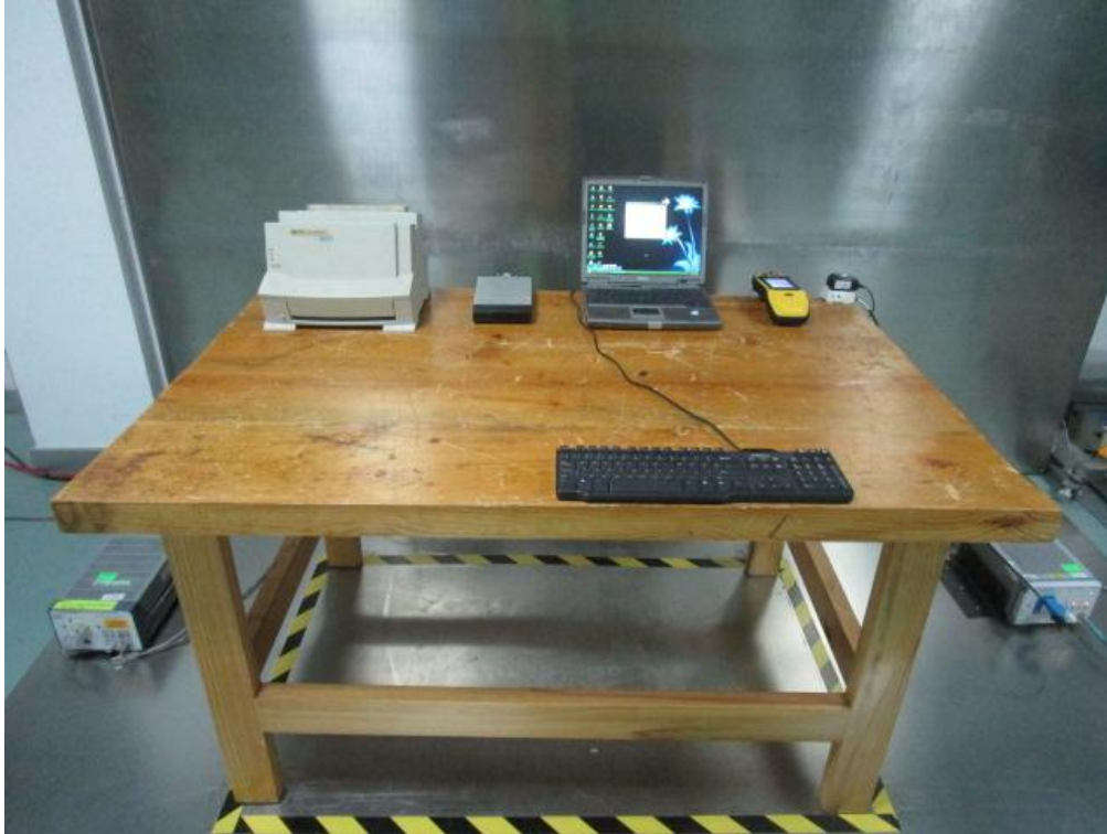
Photograph 2: Set-up for Spurious Emissions below 1GHz
