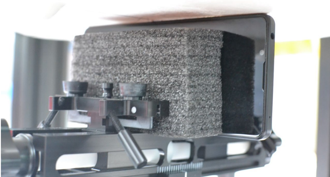
SAR Test Setup Photo 16 – Phablet, Left Side at 0mm
