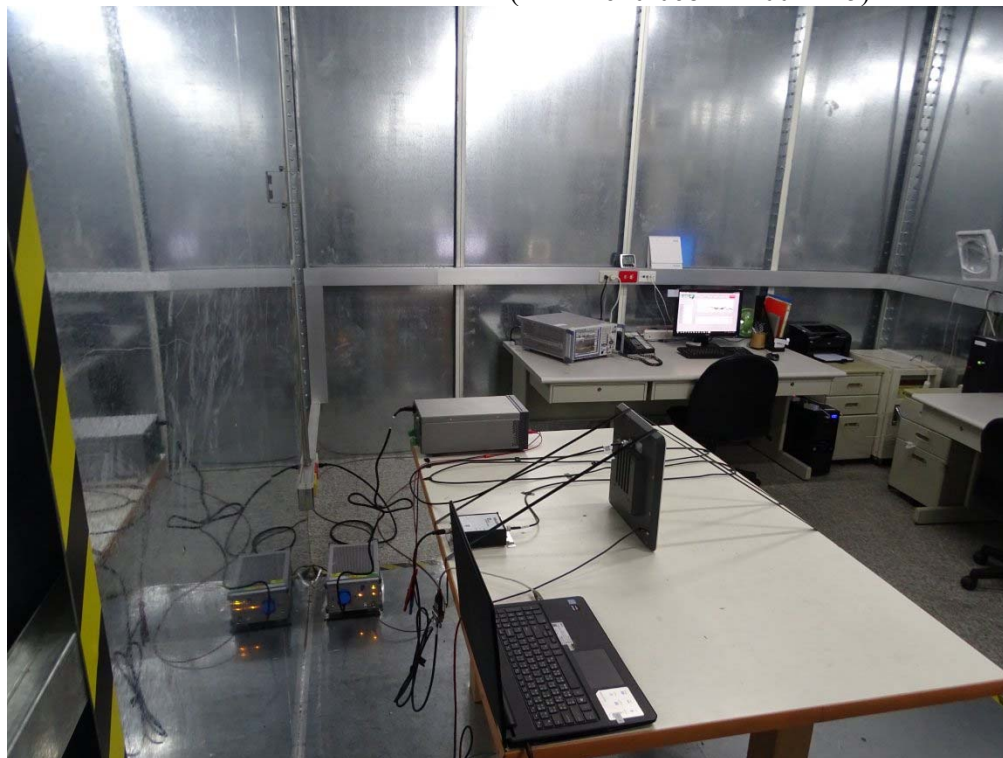
Back View of Conducted Test (BIS U-620-068-111-00-S115)
