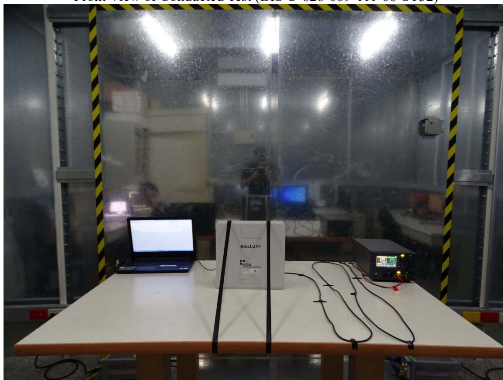
Front View of Conducted Test (BIS U-626-069-111-06-ST32)
