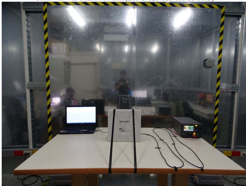
Front View of Conducted Test (BIS U-620-068-111-00-S115)
