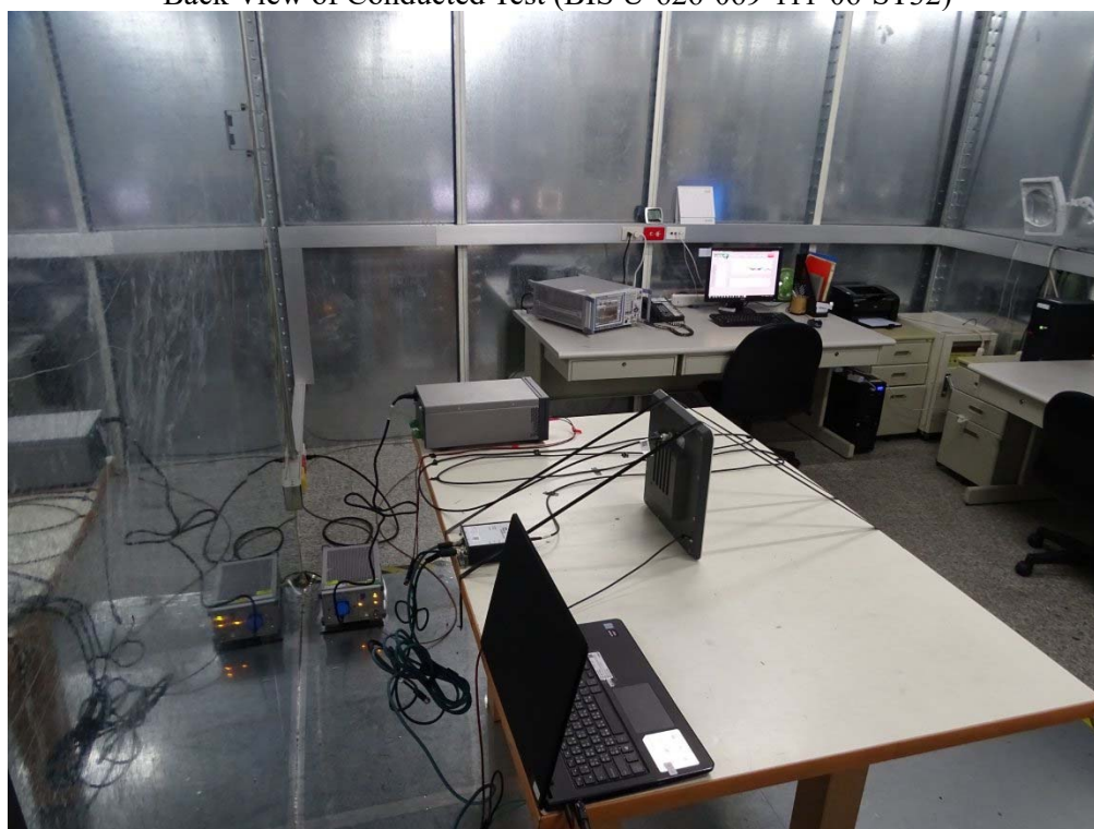
Back View of Conducted Test (BIS U-626-069-111-06-ST32)
