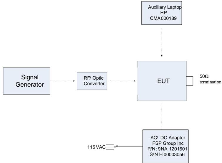
**Figure 2. Test Set-Up – Radiated**
