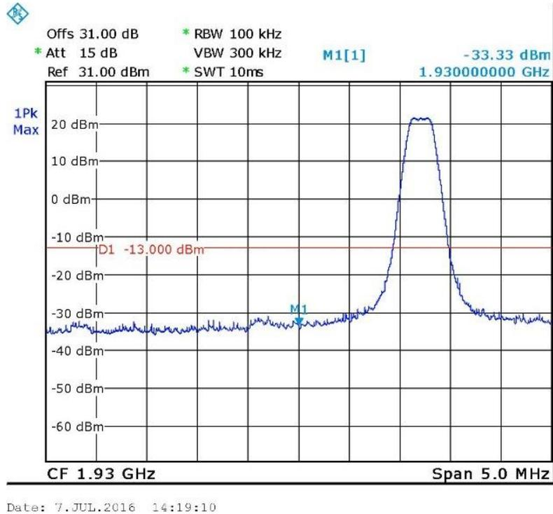
Figure 54. — GSM - 1931.2 MHz
