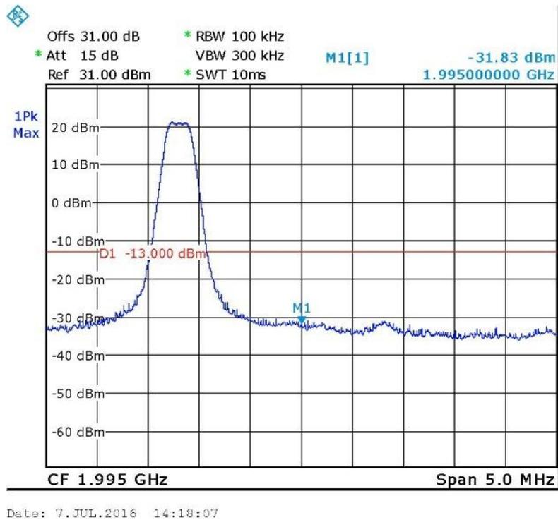
Figure 55. — GSM - 1993.8 MHz
