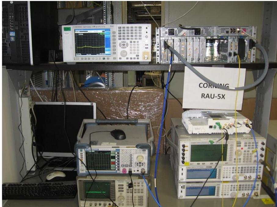
Figure 3. Conducted Emission From Antenna Port Test
