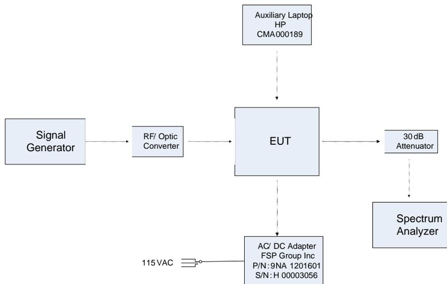
**Figure 1. Test Set-Up – Conducted**
