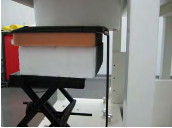
Fig.3 EUT Lap-held mode to flat phantom
