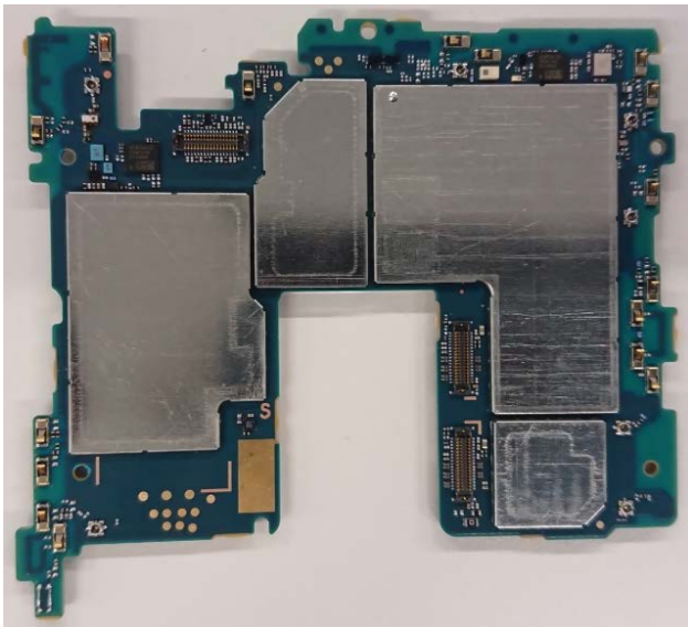
Internal PWB with Shield cases (Rear-side)
