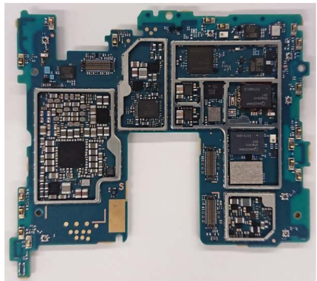
Internal PWB without Shield cases (Rear-side)
