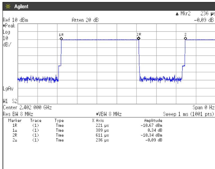
$$\text{Duty Cycle} = \text{Ton} / (\text{Ton} + \text{Toff}) = 389[\mu\text{s}] / (389[\mu\text{s}] + 236[\mu\text{s}]) = 62.24[\%]$$
