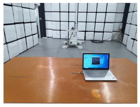
Radiated Measurement (Above 1GHz)
