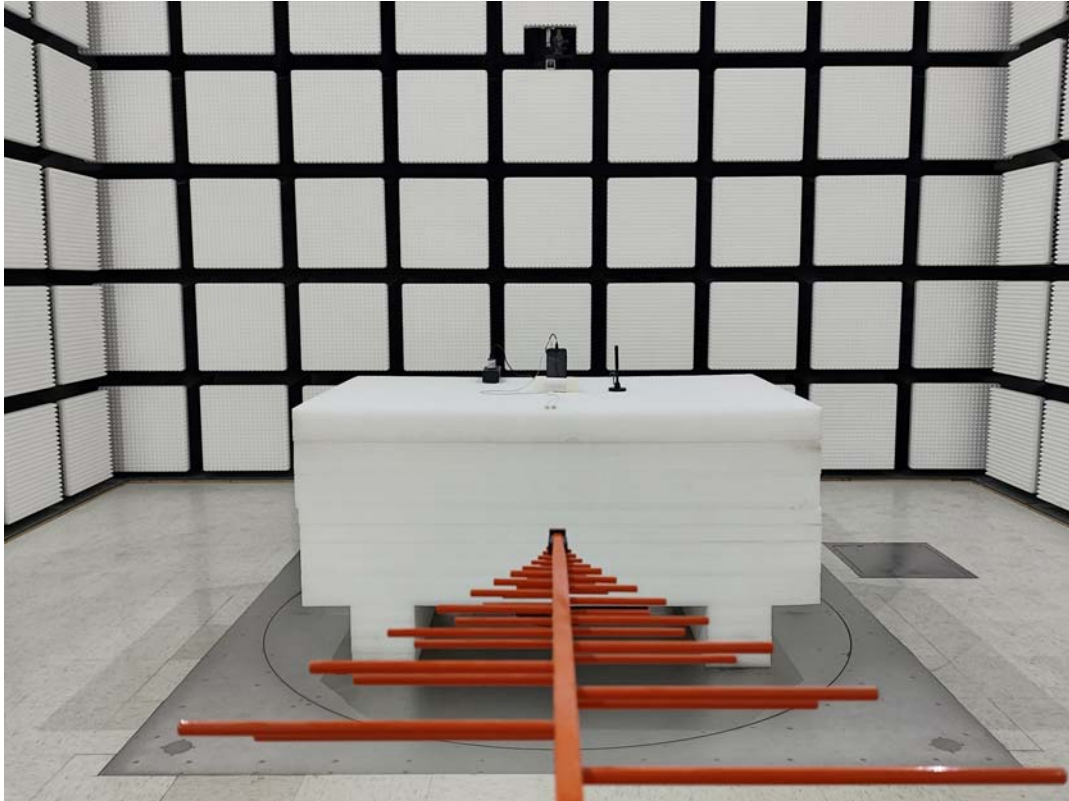
Radiated Emission Above 1GHz View
