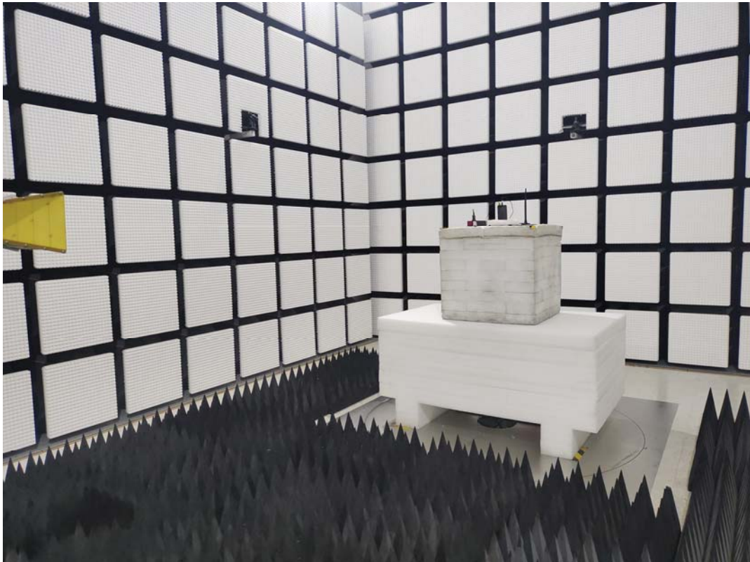
Radiated Emission Above 1GHz View
