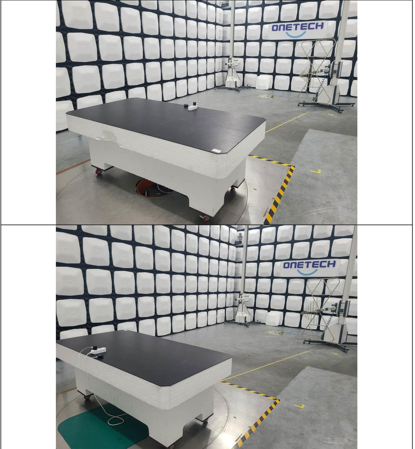
**Radiated Emission Test Set Up (Above 1 GHz)**
