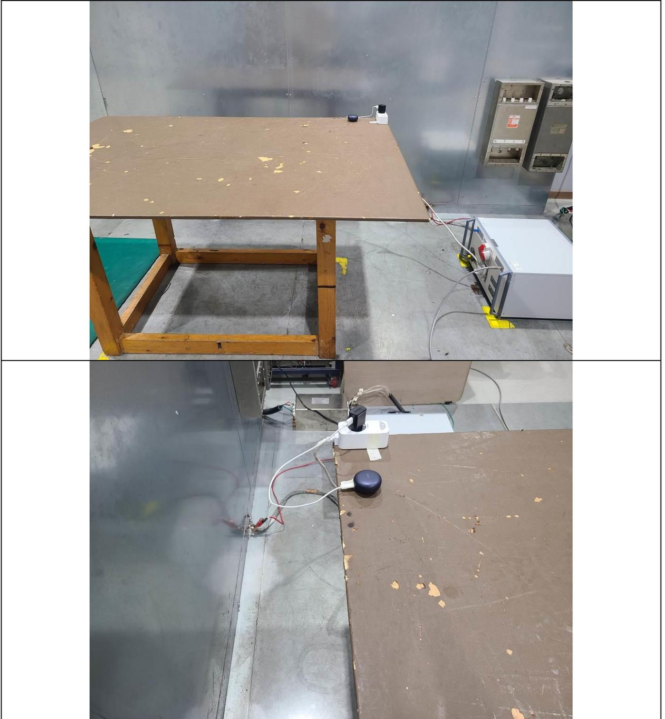
**Radiated Emission Test Set Up (Below 1 GHz)**
