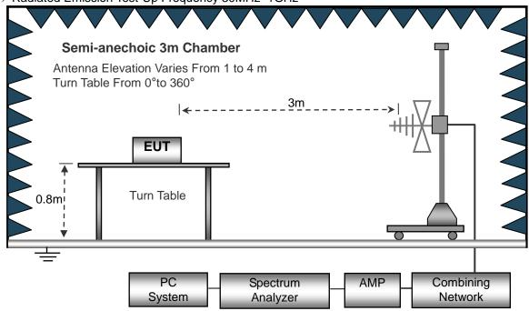
(C) Radiated Emission Test-Up Frequency Above 1GHz
