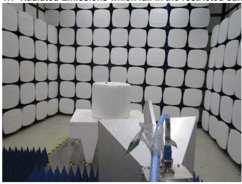
1.2 Radiated Spurious Emissions Test Setup
