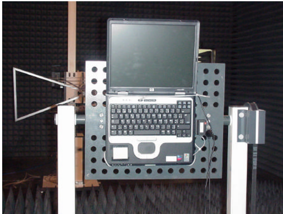
Picture 3 : Setup for radiated measurements
