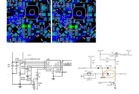
Minor changes for the LED circuit, and changed RT8498 to SY8707, the new chip is pin-for-pin compatible. This change is to facilitate the purchase of raw materials. The function and electrical characteristics have not been changed.
