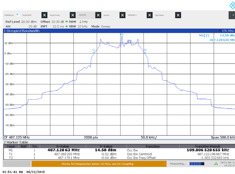
Plot 1: 487.125 MHz, max hold with frequency variation from 50 Hz to 15 kHz
