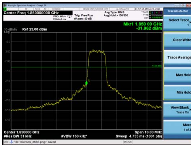
LTE Band 2 3MHz QPSK 1RB CH-Low
