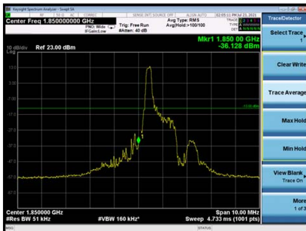
LTE Band 2 3MHz QPSK 1RB CH-Low
