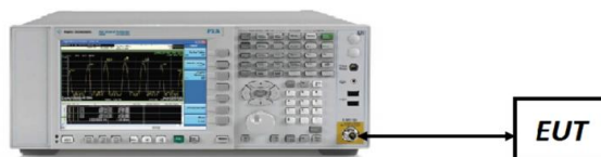
Figure 7-5. Test Instrument & Measurement Setup
