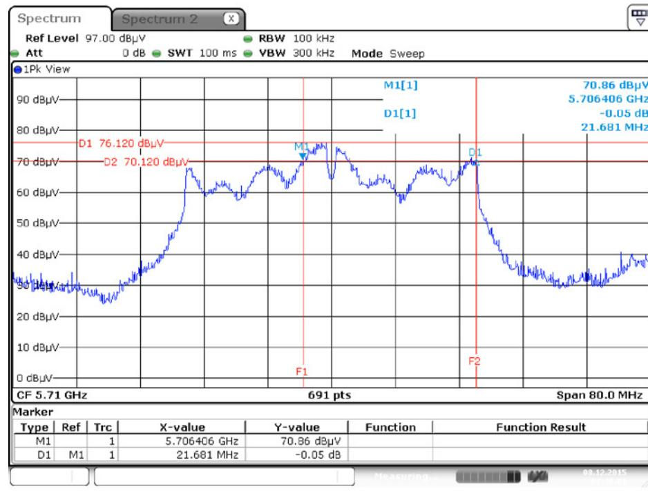
**6 dB Bandwidth Plot on Configuration IEEE 802.11ac MCS0/Nss1 VHT80 / Chain 1 + Chain 2 + Chain 3 + Chain 4 / 5690 MHz**
