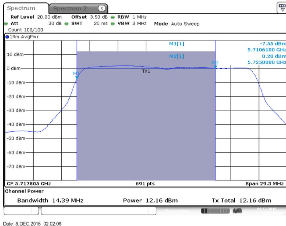
**Conducted Output Power Plot on Configuration IEEE 802.11ac MCS0/Nss1 VHT20 / Chain 2 / 5720 MHz (UNII2C)**
