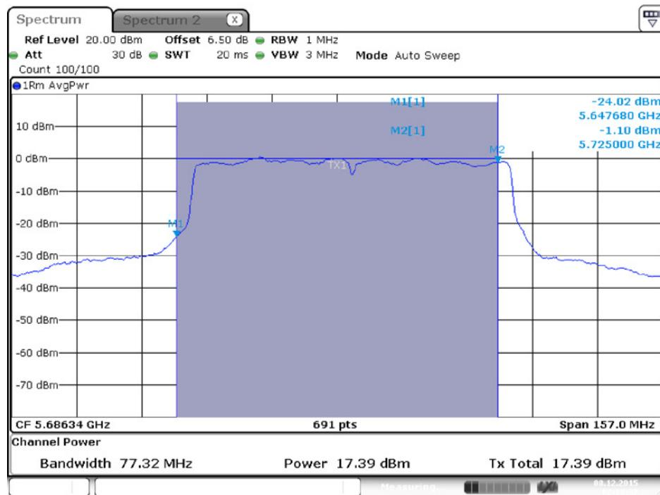
**Conducted Output Power Plot on Configuration IEEE 802.11ac MCS0/Nss1 VHT80 / Chain 3 / 5690 MHz (UNII2C)**
