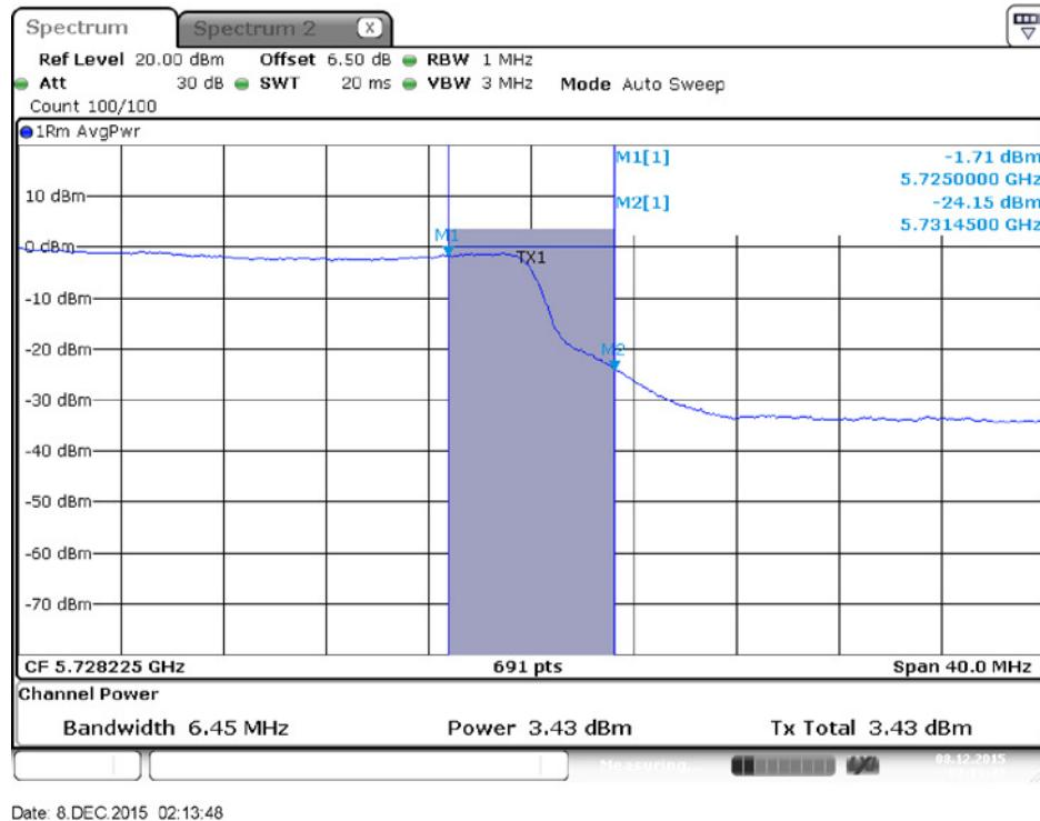
**Conducted Output Power Plot on Configuration IEEE 802.11ac MCS0/Nss1 VHT80 / Chain 4 / 5690 MHz (UNII 3)**
