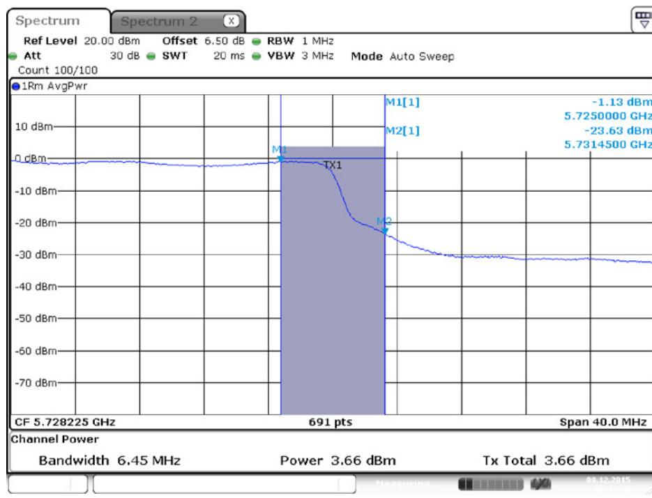
**Conducted Output Power Plot on Configuration IEEE 802.11ac MCS0/Nss1 VHT80 / Chain 3 / 5690 MHz (UNII 3)**
