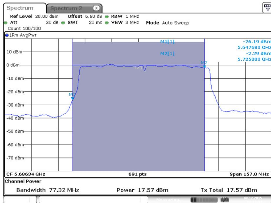
**Conducted Output Power Plot on Configuration IEEE 802.11ac MCS0/Nss1 VHT80 / Chain 1 / 5690 MHz (UNII 3)**
