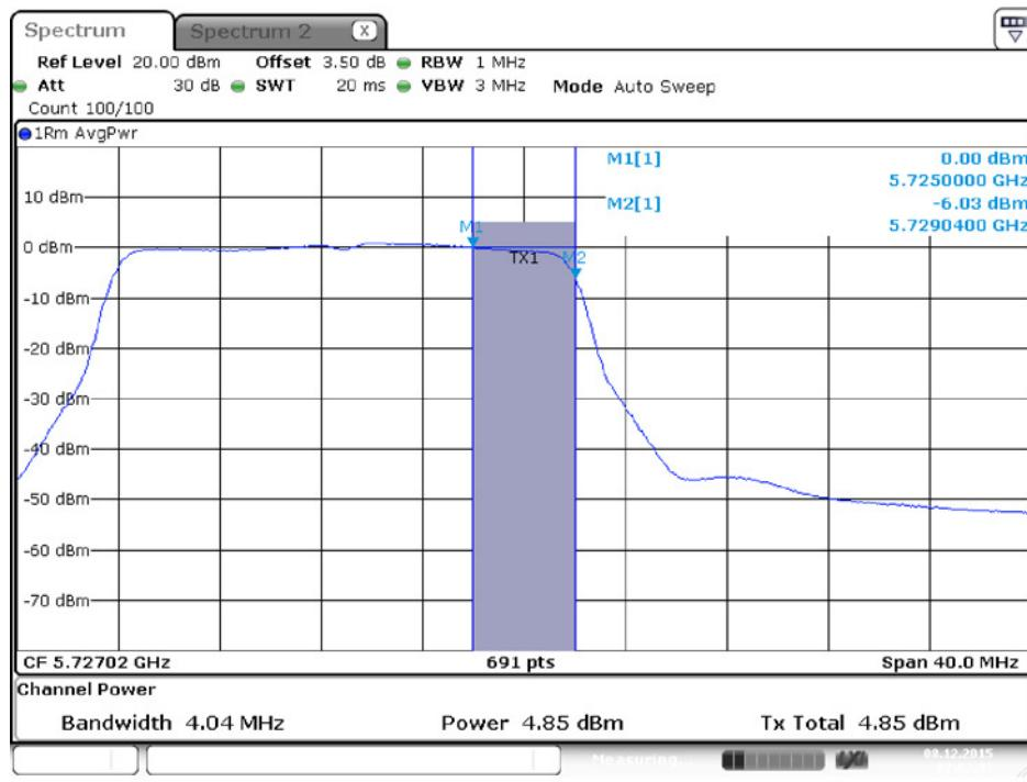
**Conducted Output Power Plot on Configuration IEEE 802.11ac MCS0/Nss1 VHT40 / Chain 1 / 5710 MHz (UNII2C)**
