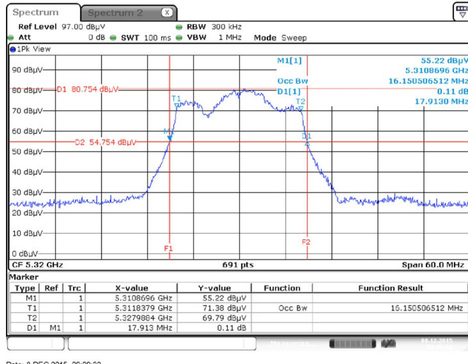
**26dB Bandwidth and 99% Occupied Bandwidth Plot on Configuration IEEE 802.11a / Chain 1 +
