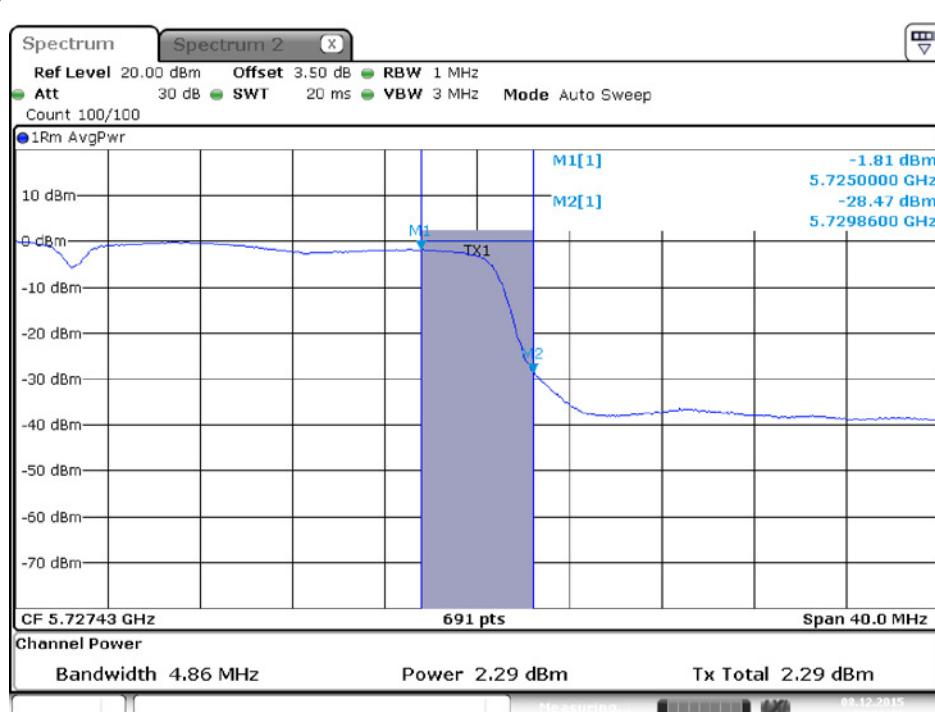
**Conducted Output Power Plot on Configuration IEEE 802.11ac MCS0/Nss1 VHT40 / Chain 3 / 5710 MHz (UNII 3)**
