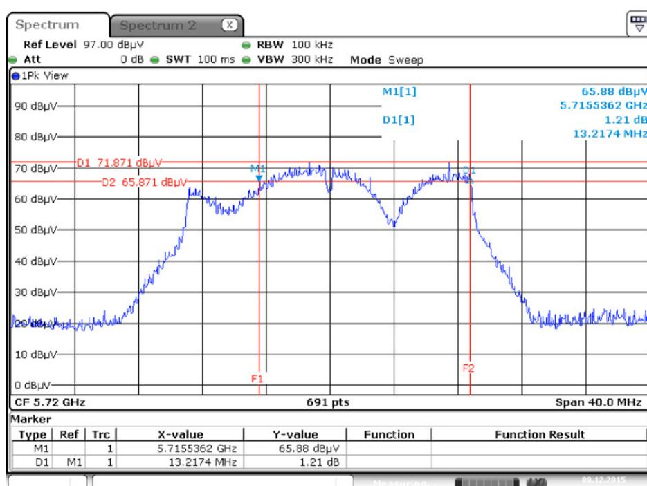
**6 dB Bandwidth Plot on Configuration IEEE 802.11ac MCS0/Nss1 VHT40 / Chain 1 + Chain 2 + Chain 3 + Chain 4 / 5710 MHz**
