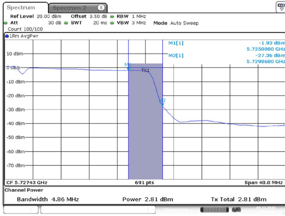
**Conducted Output Power Plot on Configuration IEEE 802.11ac MCS0/Nss1 VHT40 / Chain 4 / 5710 MHz (UNII 3)**
