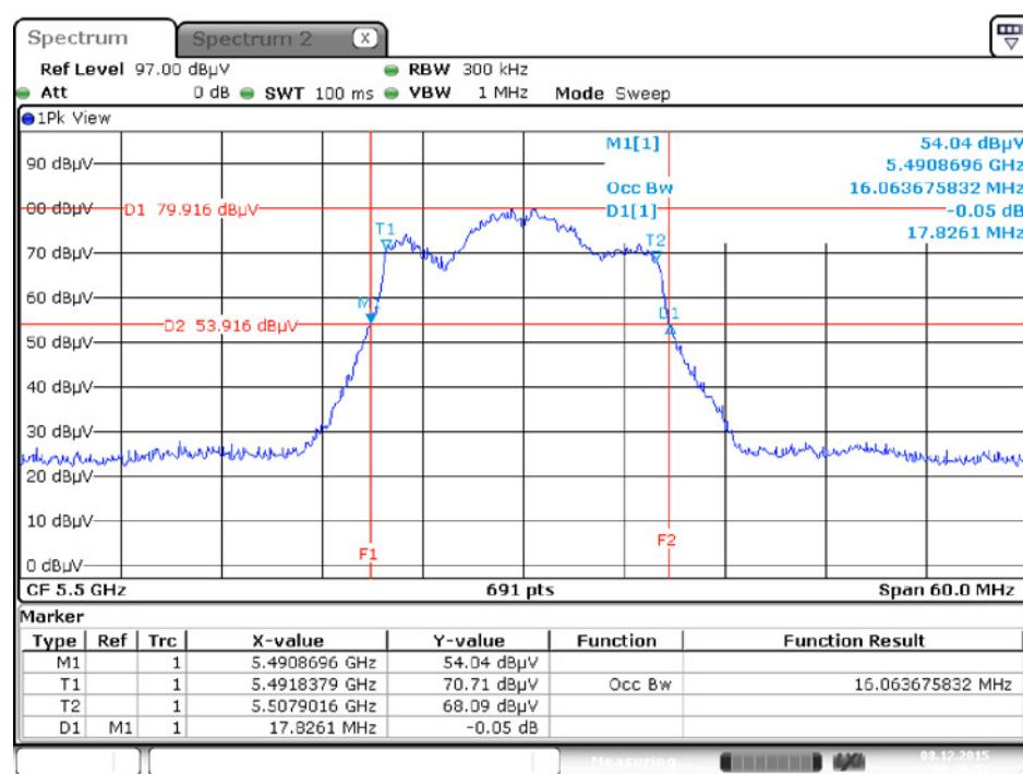
**26dB Bandwidth and 99% Occupied Bandwidth Plot on Configuration IEEE 802.11a / Chain 1 +
