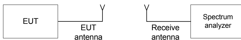
Figure 7.1.1 The 20 dB bandwidth test setup
