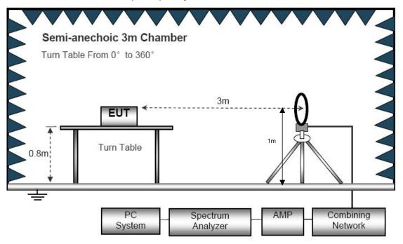
(B) Radiated Emission Test-Up Frequency 30MHz~1GHz
