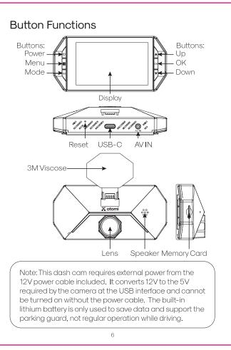
Under the shutdown state, press to power ON. In the startup state, long press to power OFF and short press to open/close the display.
