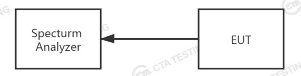
The EUT is connected to the Spectrum Analyzer; the RF load attached to the EUT antenna termina is 50 Ohm; the path loss as the factor is calibrated to correct the reading. Make the measurement with the spectrum analyzer's resolution bandwidth(RBW) = 100 kHz. In order to make an accurate measurement, set the span greater than RBW.
