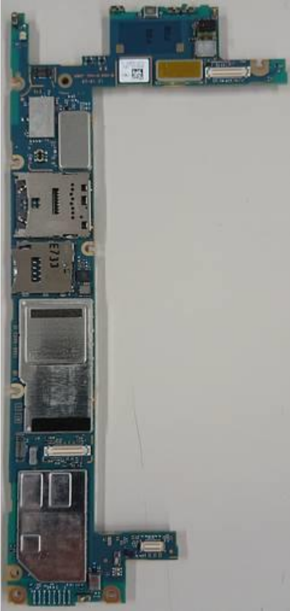
Internal PWB with Shield cases (Front-side)
