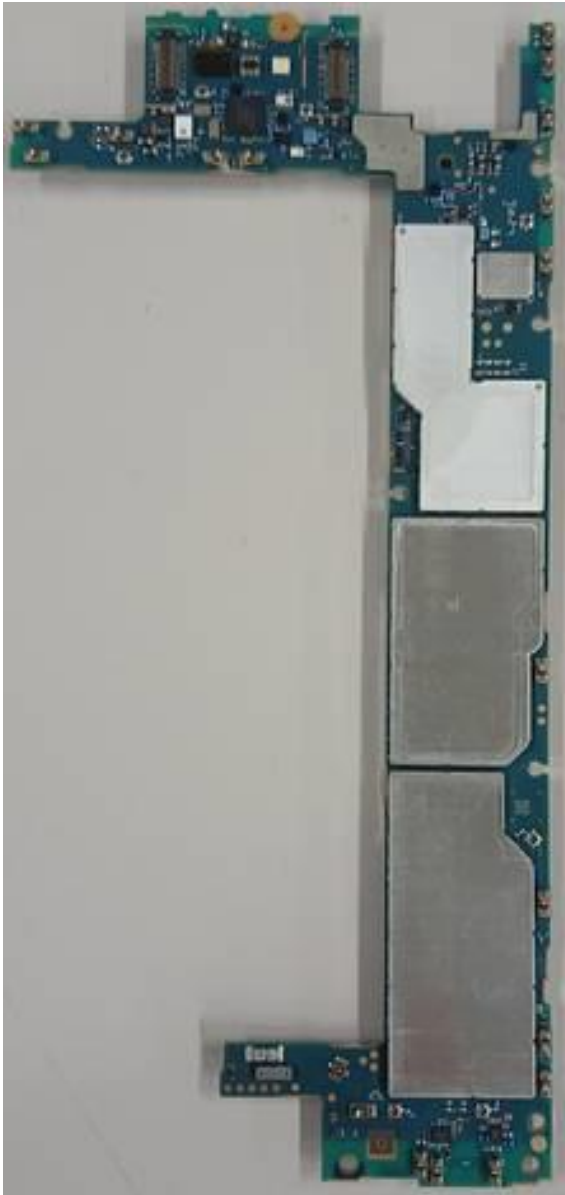
Internal PWB with Shield cases (Rear-side)
