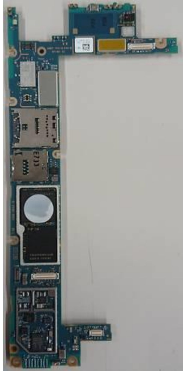
Internal PWB without Shield cases (Front-side)
