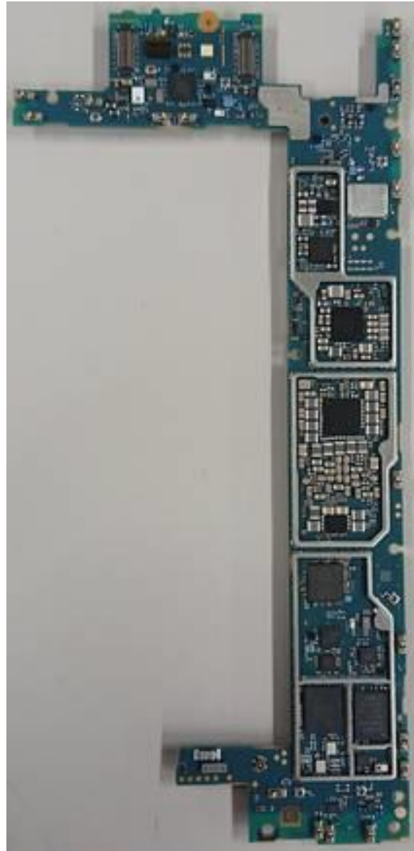
Internal PWB without Shield cases (Rear-side)
