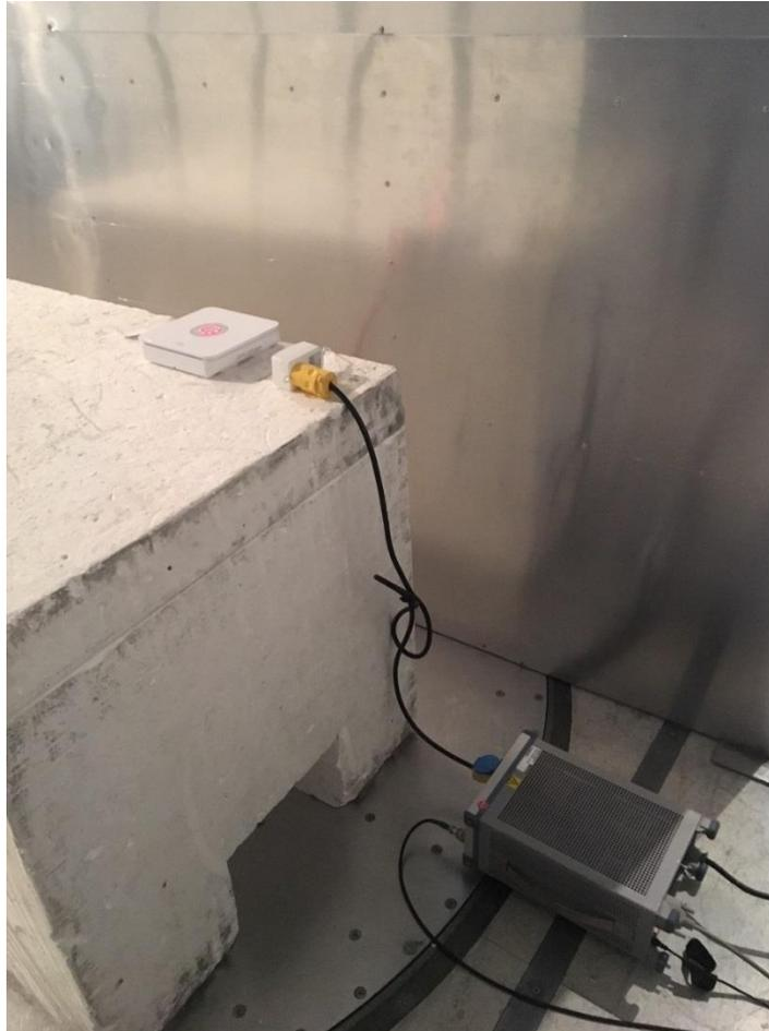
*Figure 1.2-1: AC power line conducted emissions – setup photo*
