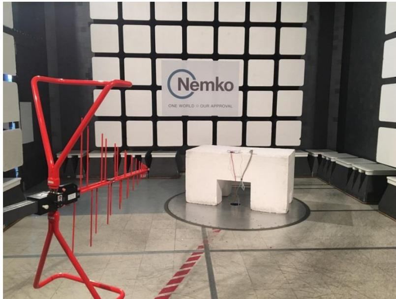
*Figure 1.1-1: Radiated emissions setup photo – below 1 GHz*
