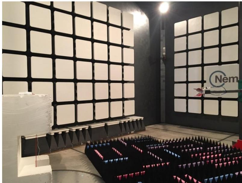
*Figure 1.1-3: Radiated emissions setup photo – above 1 GHz*
