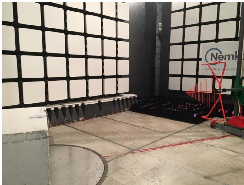
*Figure 1.1-2: Radiated emissions setup photo – below 1 GHz*
