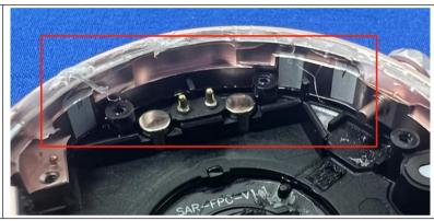
The antenna is Metal frame antenna.
