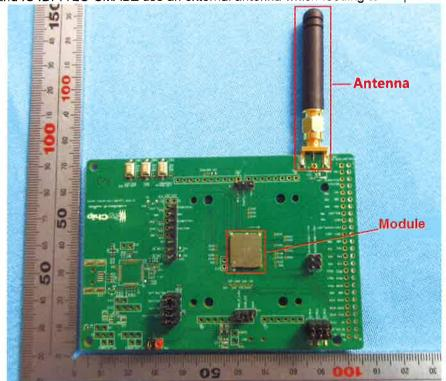
We apply for Limited Modular Transmitter Approval because the module doesn't fulfil the antenna condition as described above. A compressed whip antenna (ANT-SS900 from LPRS, gain=1.04dBi) was adopted to perform the radiated tests of Limited Modular Transmitter Approval.
