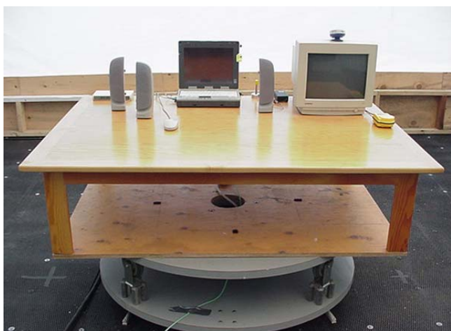
Photograph F.7-3 - Front of Radiated Emission Setup
