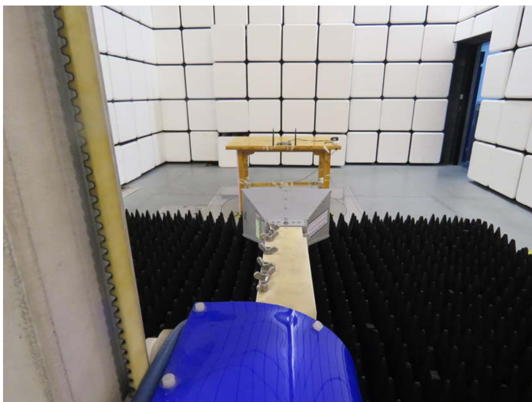
Picture 2: Radiated Spurious Emissions Test setup
