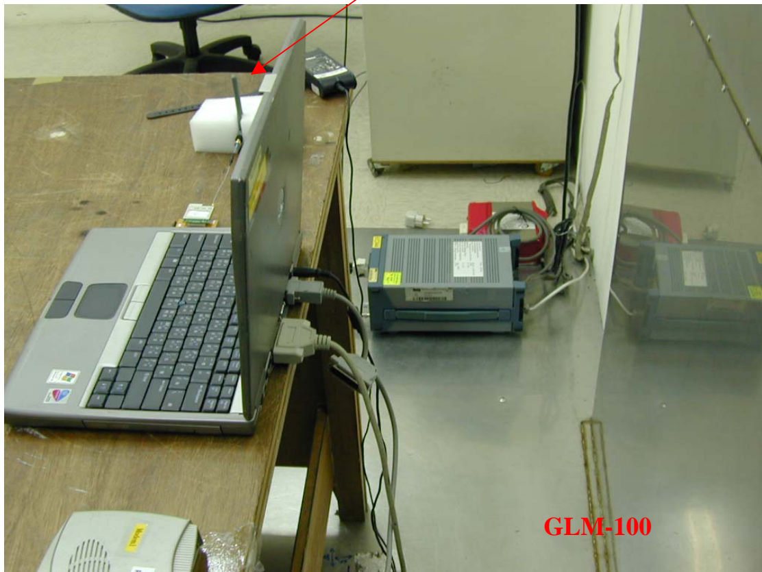
Photo 2: Conducted Emission Test set-up photo (Dipole Antenna)
