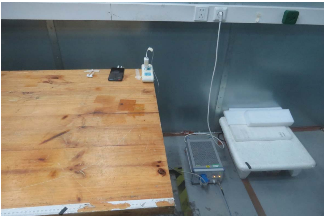
Picture 2 Conducted Emission Test Setup
