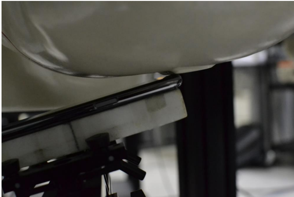
SAR Test Setup Photo 4 – Left Tilt
