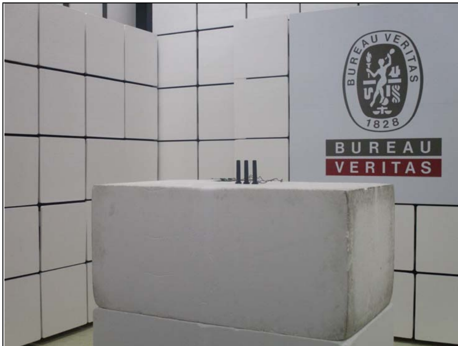
Radiated Emission Test (Above 1GHz)
