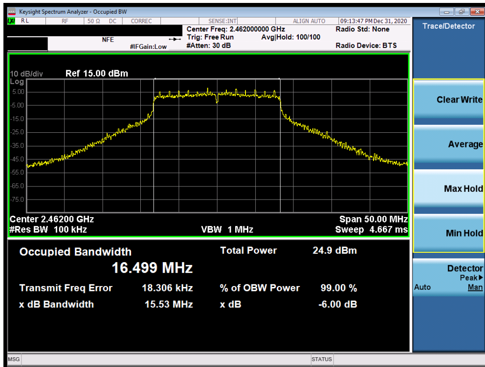
Plot 7-6. 6dB Bandwidth Plot (802.11g – Ch. 11)
