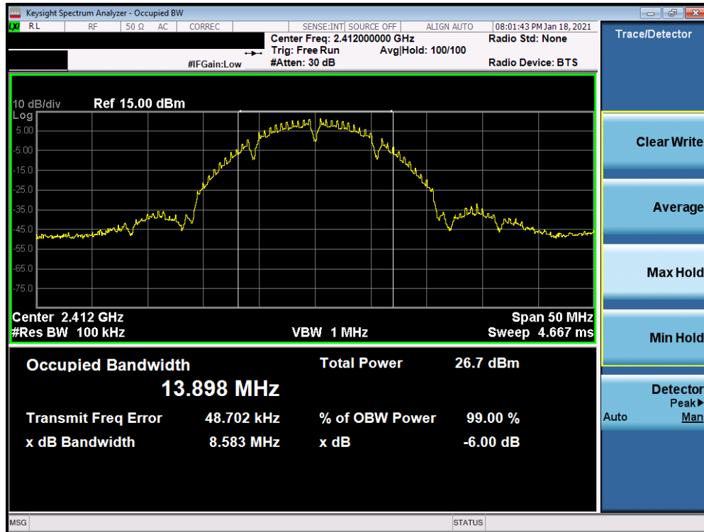
Plot 7-1. 6dB Bandwidth Plot (802.11b – Ch. 1)
