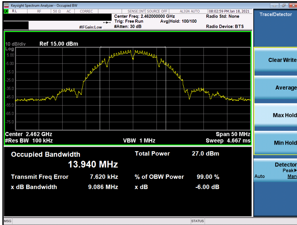
Plot 7-3. 6dB Bandwidth Plot (802.11b – Ch. 11)
