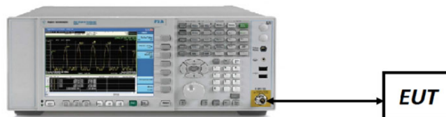
Figure 7-1. Test Instrument & Measurement Setup
