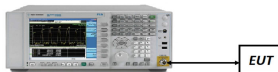
Figure 7-5. Test Instrument & Measurement Setup
