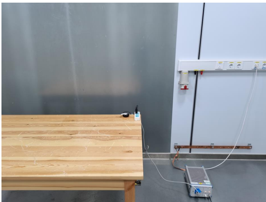
Fig. 4 Power line conducted emission setup photo
