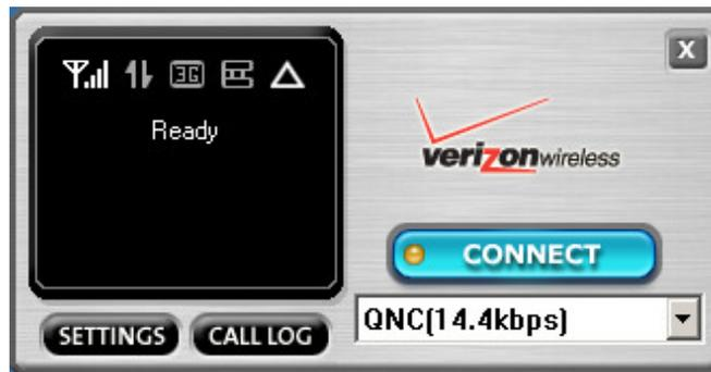
The Main Window provides access to the status of the SCP-500®, Data Service Connection, and Menu for accessing more features.
