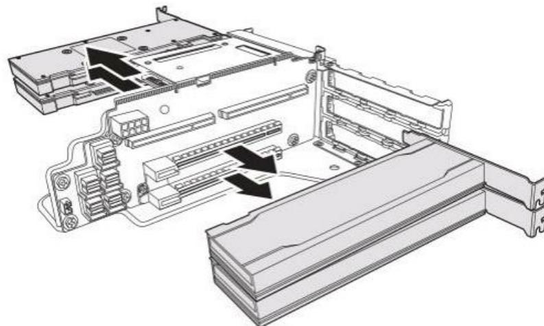
**Figure 1-45: Removing the Tesla T4 Cards**
