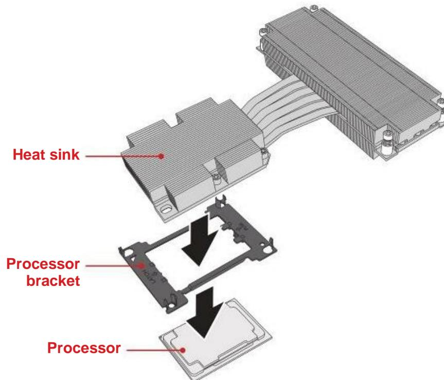
**Figure 1-58: Removing the Processor**
