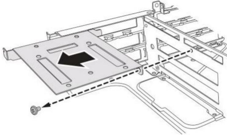
**Figure 1-53: Removing the SSD Tray**
