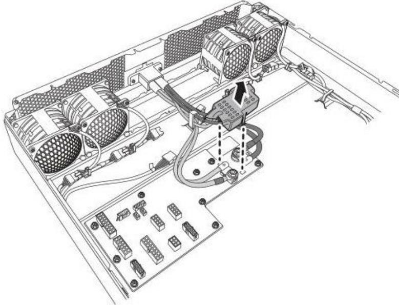
**Figure 1-15: Removing the Cable Protective Cap**
