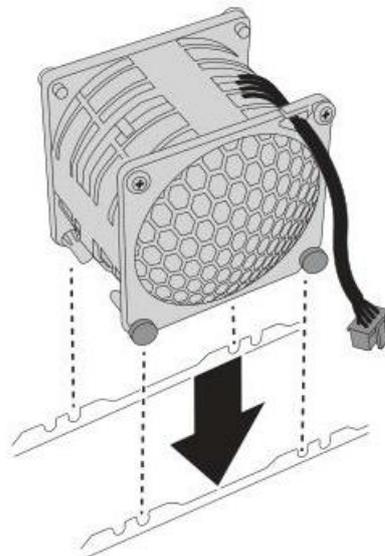
**Figure 1-12: Installing the Fan Module Assembly**
