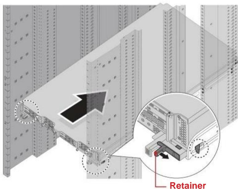
**Figure 2-3: Installing the Server in the Rack**
