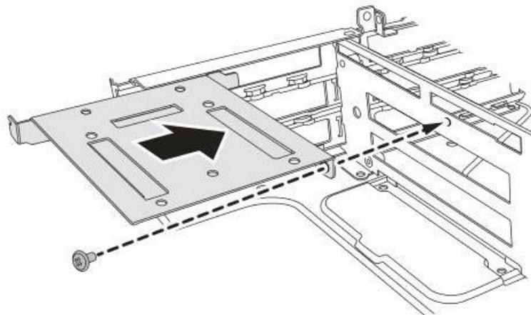
**Figure 1-54: Installing the SSD Tray**
