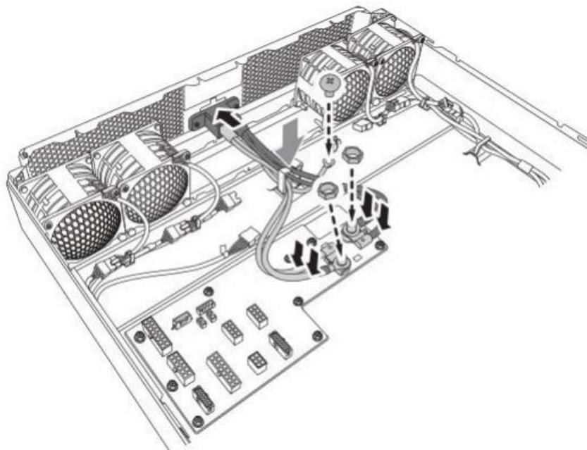
**Figure 1-20: Installing the Busbar Power Cables**
