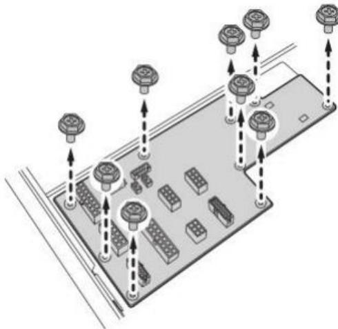
**Figure 1-18: Removing the PDB Board**
