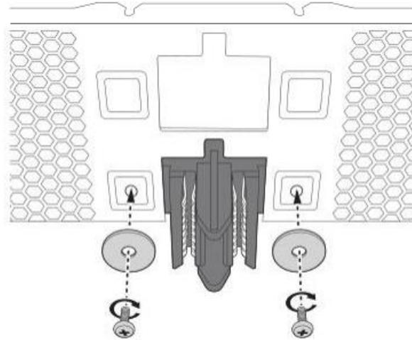
**Figure 1-21: Installing the the Screws and Washers**
