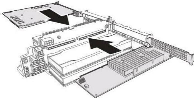
**Figure 1-37: Installing the K2T-QB and K2C-AB Cards**
