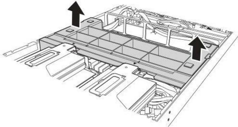
Figure 1-6: Removing the Air Duct
