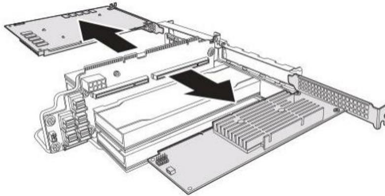
**Figure 1-34: Removing the K2T-QB and K2C-AB Cards**
