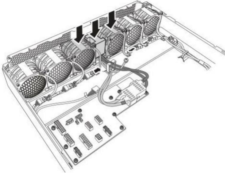
**Figure 1-23: Installing the Fan Modules and Rubber Pad**
