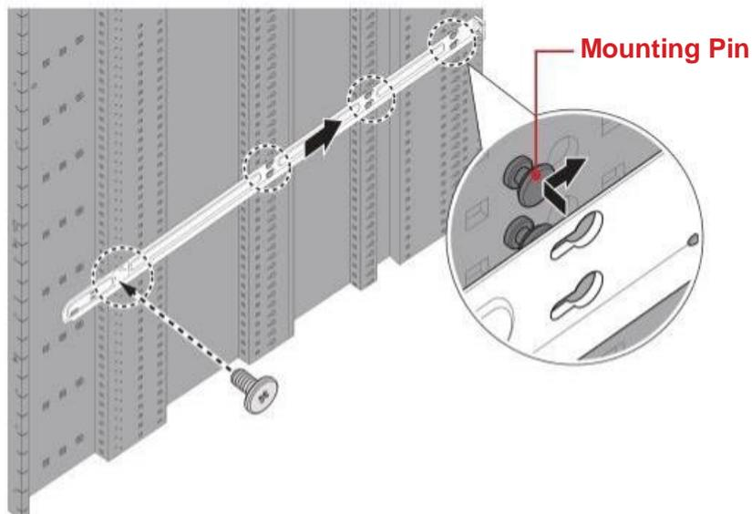
**Figure 2-1: Installing the Left Rail**
