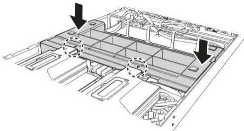
Figure 1-7: Installing the Air Duct
