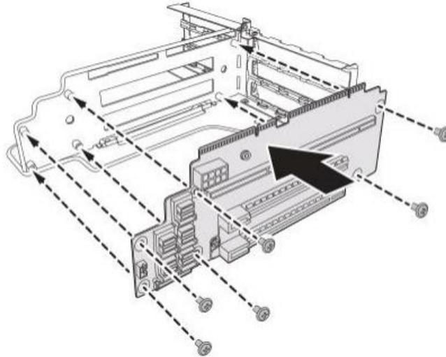
**Figure 1-41: Installing the Riser 1 Board**
