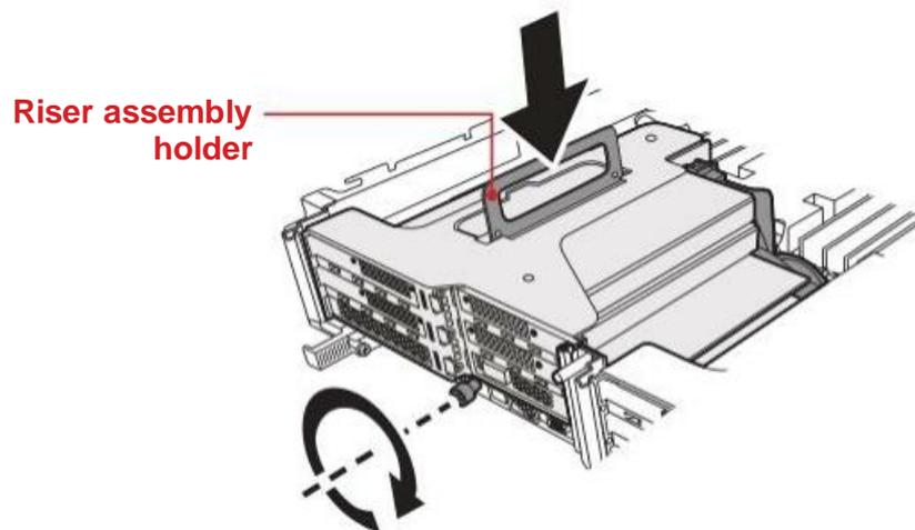
**Figure 1-49: Installing the Riser 2 Assembly**
