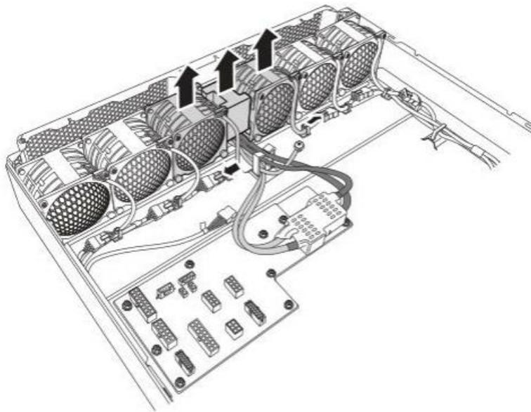
**Figure 1-14: Removing the Fan Modules and Rubber Pad**
