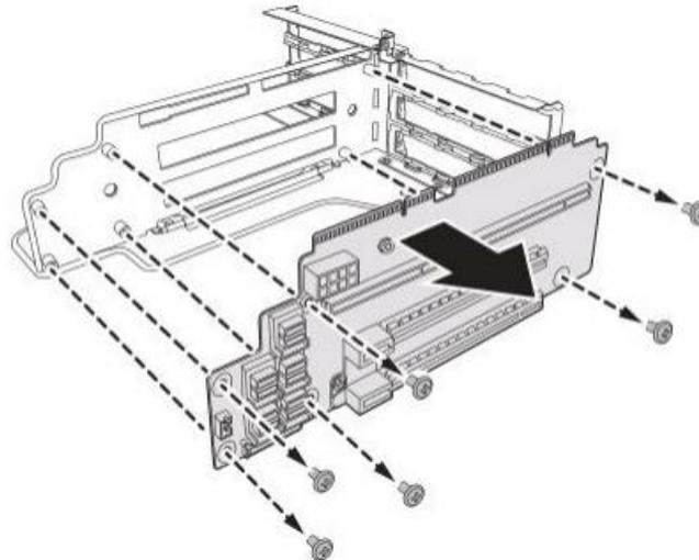
**Figure 1-40: Removing the Riser 1 Board**
