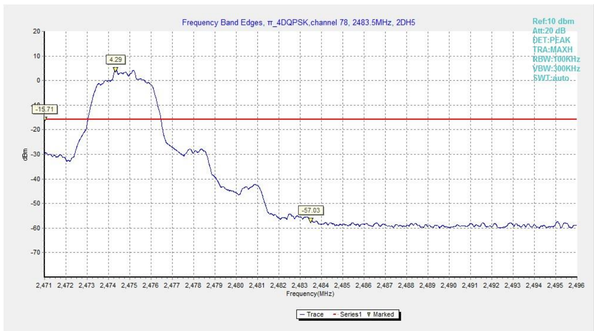
Fig. 10 Band Edges ( \pi/4 DQPSK, Ch 78, Hopping OFF)
