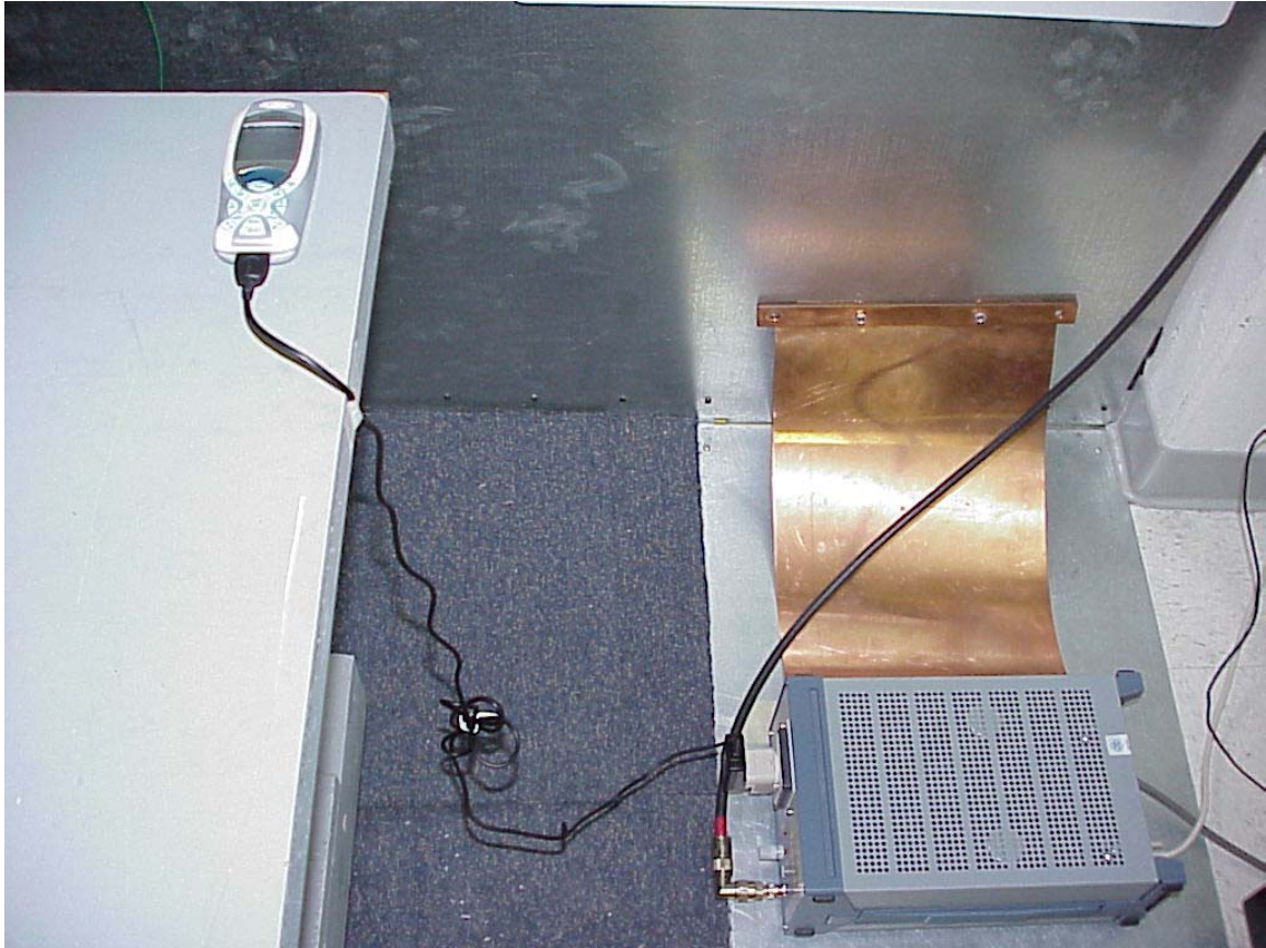
Test setup – AC Line Conducted Emissions
