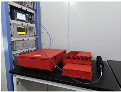
Radiated Spurious Emissions (30MHz-1GHz)
