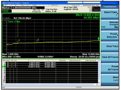
Tx Spurious Emissions 1GHz-10GHz. BLE 2442MHz average vertical
