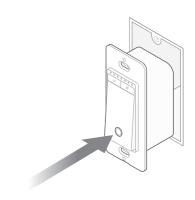
6 Attach the wallplate and turn on the circuit breaker. Then the wiring is finished.
