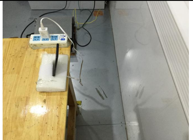
Conducted Emissions Test Setup Side View
