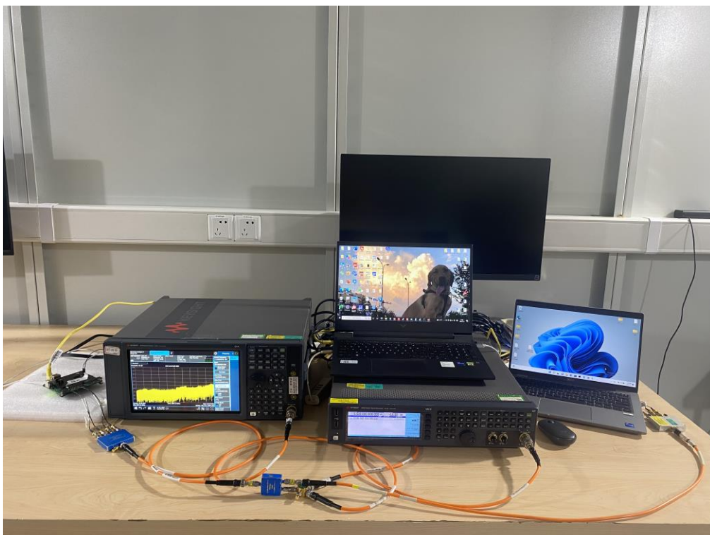
Description: DFS Test Setup
