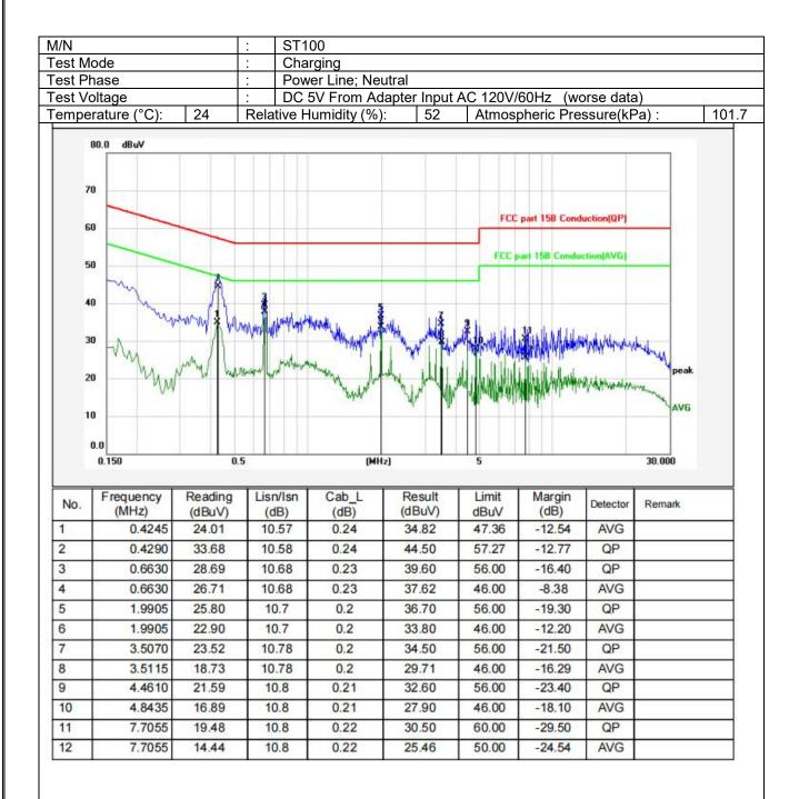
Remarks: 1. Result=Reading+Lisn+Cab\_L 2. If the average limit is met when using a quasi-peak detector. the EUT shall be deemed to meet both limits and measurement with average detector is unnecessary.
