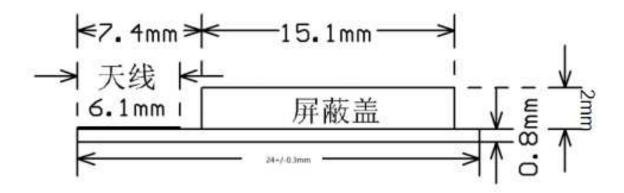
Note: The default dimensional tolerance is 0.3 mm. If you have specific requirements on dimensions, make them clear in the datasheet after communication.
